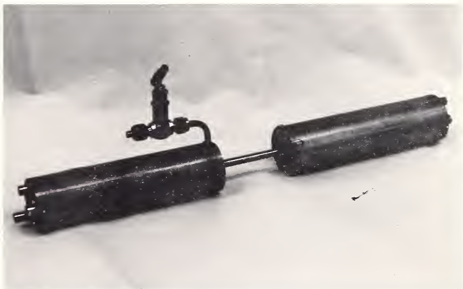
FIGURE 2. High-resolution position sensitive neutron detector. The detector region is the center small-diameter tube. Special amplifiers are enclosed in the large-diameter cylinders at each end. The valve allows the gas used in the ionization chamber to be changed to determine the effects of different mixtures and pressures. The detector is presently operating with a mixture of 3.1 \times 10^5 pascals of ^3\text{He} , 7.9 \times 10^5 pascals of xenon and 0.4 pascals of carbon dioxide. ( 10^5 pascal \cong 1 atmosphere).
