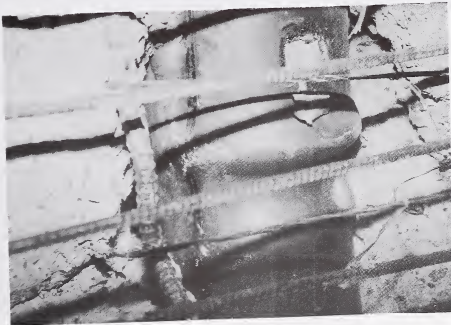
Photograph 2. Fracturing of Steel Pipe
