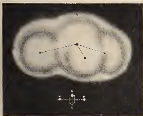
The atomic clock (top) developed by the Bureau (p. 66) provides a new primary standard of frequency and time invariant with age. Lower left: drawing of the ammonia molecule whose microwave absorption line (lower right) provides the invariant frequency that controls the timekeeping of the clock. The ammonia gas is maintained in the 30-ft absorption cell wound around the synchronous clock above the panel.
