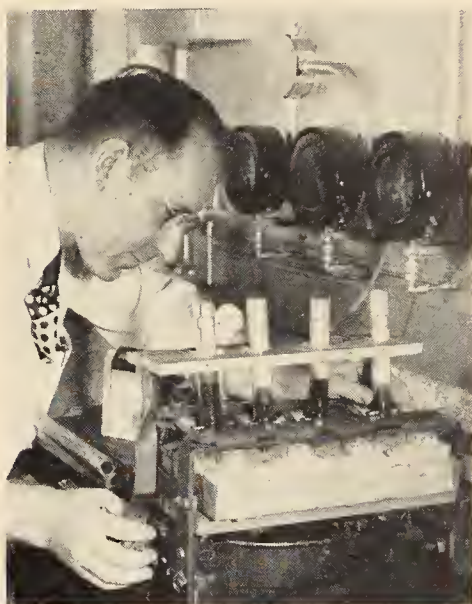
Left: water penetration of leather impregnated with rubber by the Bureau's new process is tested dynamically by means of a specially designed machine. Right: the increased durability of the rubber-impregnated leather is shown by a service test in which the plain leather sole was worn away twice as much as the impregnated one (p. 43).
