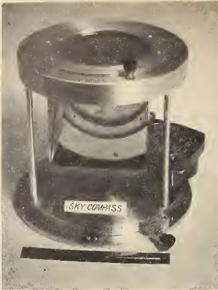
Left: the Pfund Sky Compass developed by the Bureau for use in polar regions where the magnetic compass is ineffective for navigation (p. 35). Right: a hot-wire anemometer for measurement of air speed is adjusted in the test section of the Bureau's 4½-foot wind tunnel (p. 37).
