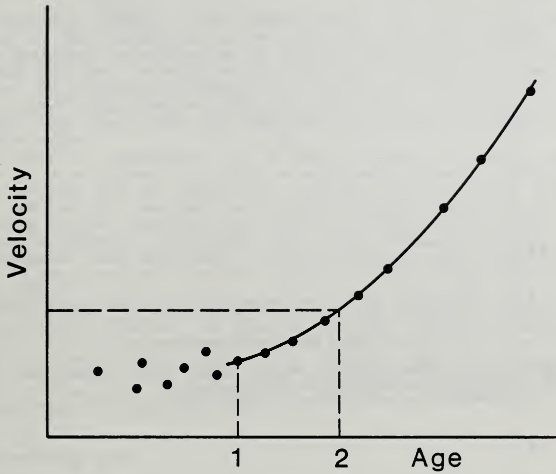
Figure 4.25 Two approaches for using impact-echo velocity measurements for defining the setting time of concrete
