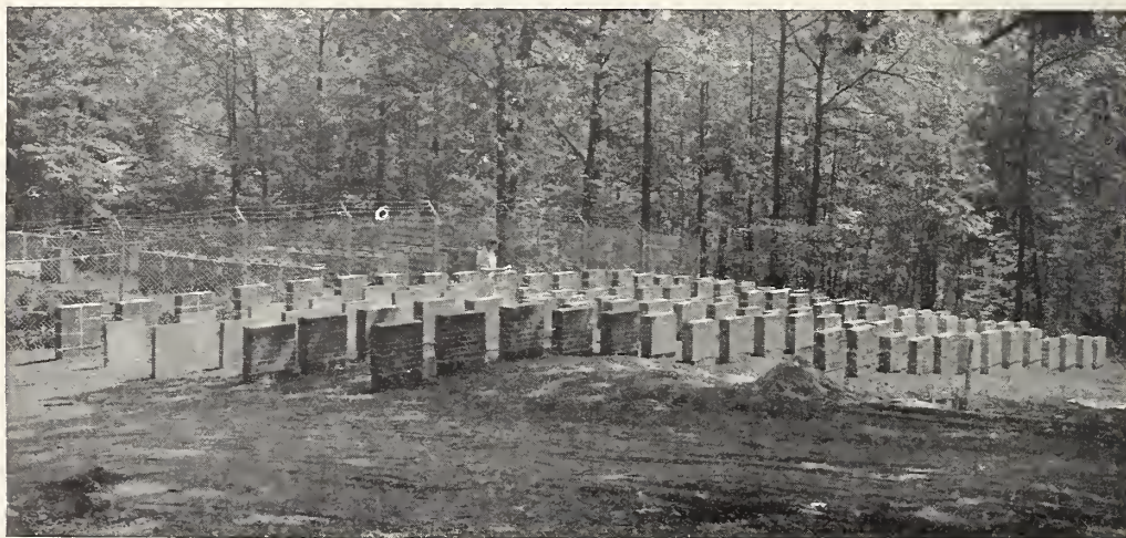
FIGURE 1.—A portion of the test field showing the position of the walls.
