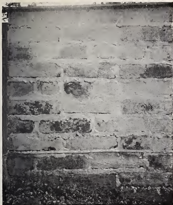
FIGURE 14.—Specimen of used common brick to which two coats of cement-water paint were applied directly.
