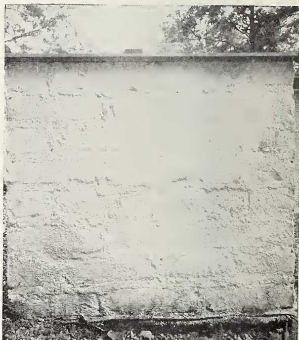
FIGURE 13.—Specimen of used common brick to which two coats of rubber-base solution-type paint were applied over grout.
