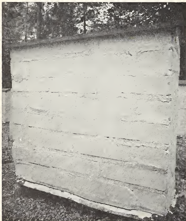
FIGURE 3.—Specimen of new common brick painted with two coats of commercial cement-water paint.
