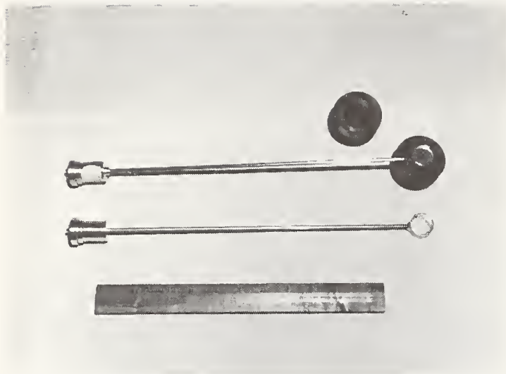
FIG. 1. NBS FISSION CHAMBER WITH AND WITHOUT BORON-10 COVER
