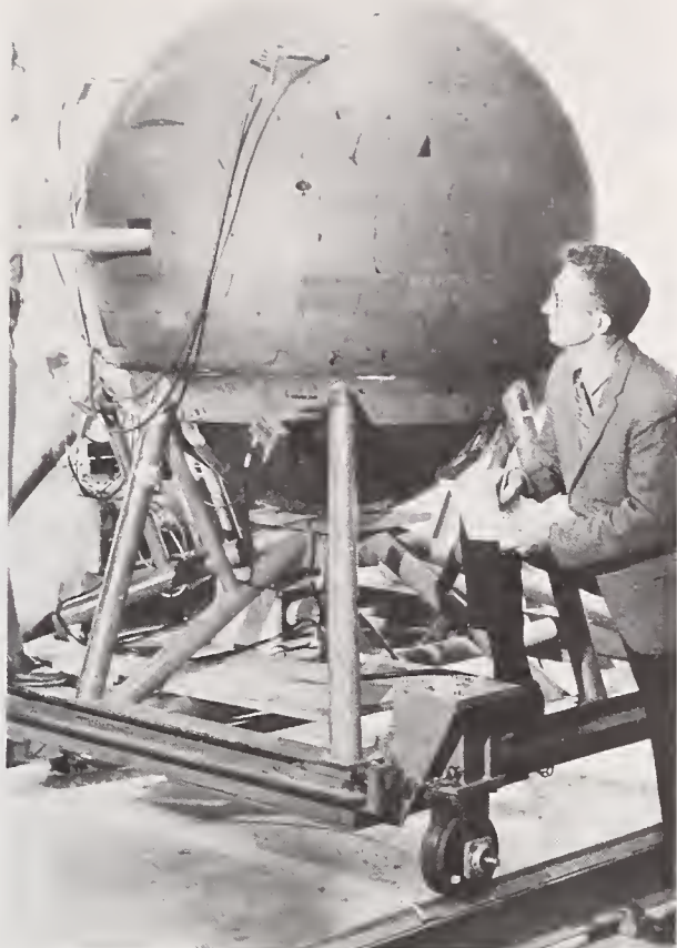
Fig. 1. The Macklin Graphite Sphere neutron Detector with C.H. Johnson at the Oak Ridge National Laboratory.
