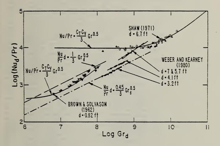
Figure 4. Comparison of experimental results for convection through openings in vertical partitions [12]
