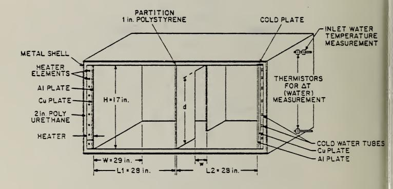
Figure 3. Two-room model for determining natural convection transfer through the doorway [11]
