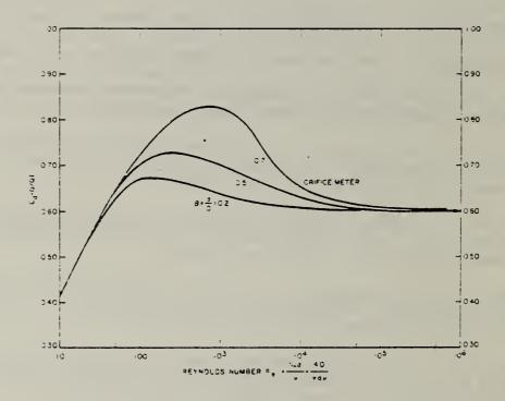
Figure 1. Orifice flow meter coefficients [6]
