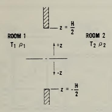
Figure 2. Schematic of opening in a vertical partition
