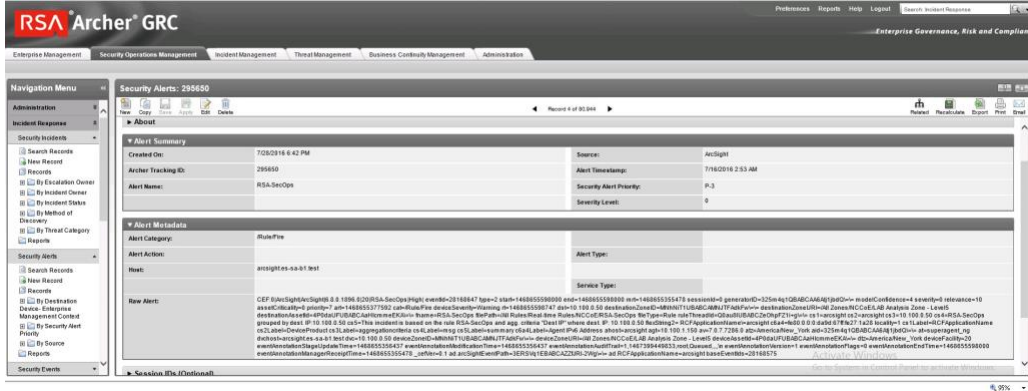
Figure 2-25 Sample Message from ArcSight, Showing Raw Log Message/Alert and Parsing with Normalization
