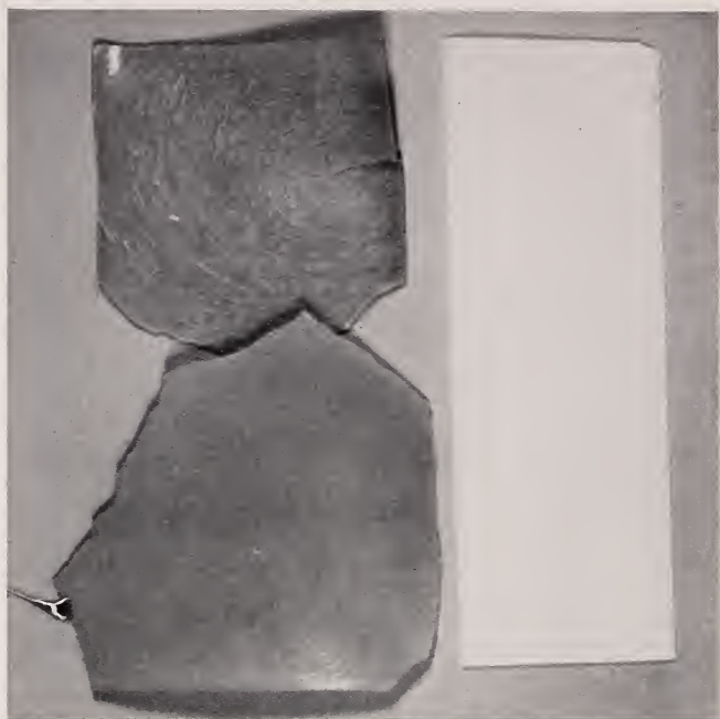
FIGURE 9.7. Samples of polyethylene aged 3 years outdoors compared with the original.
