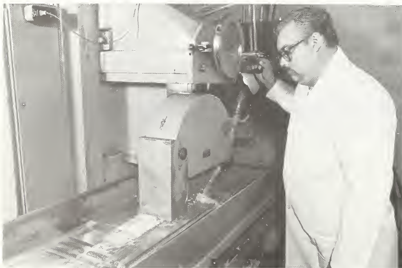
The surface grinding Frank Mills is doing removes saw marks and finishes the sizing of metal disks for x-ray and spectrometric analysis.
