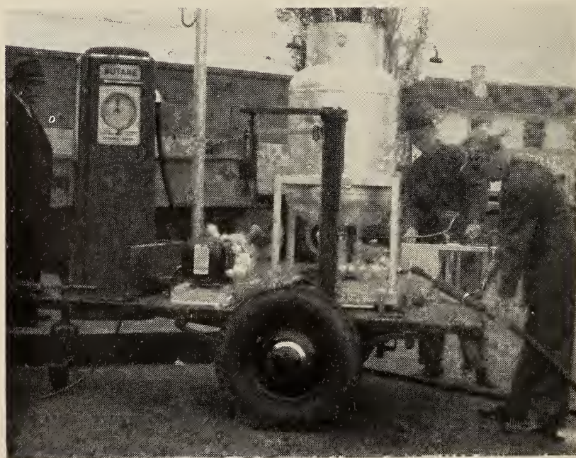
FIGURE 6.— Testing liquefied petroleum-gas meter installations in the field.
