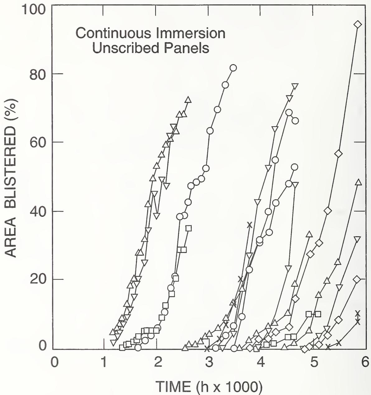
Figure 7. Percent Area Blisters Versus Immersion Time for Twenty-Four Coated Steel Panels With No Intentionally Induced Defects. The Panels Were Continuously Immersed in a 5% NaCl Solution. Six of the Twenty-Four Panels Displayed No Degradation After 6000 h of Immersion; Data for These Panels are not Displayed [Taken from Martin et al., 1990].
