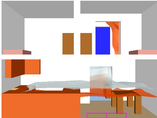
Figure 6.8: Stereo pair view of a townhouse kitchen fire. To aid in viewing the stereo effect, place a finger in front of each image. Relax your eyes allowing your two fingers and stereo pair images to merge into one.
