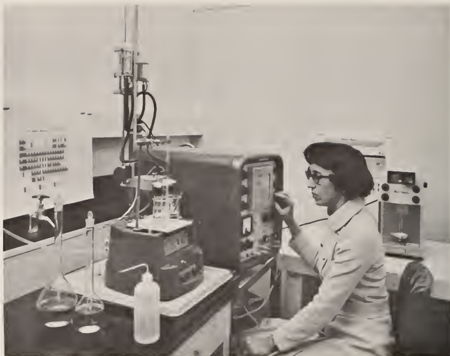
Figure 3. Apparatus used for EDTA determination.
