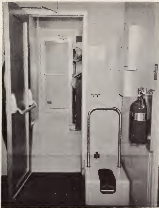
Figure 21. Anteroom, change room, and air shower. The change room is equipped with wash basin and hand drier. The pass-through is also located in the change room.
