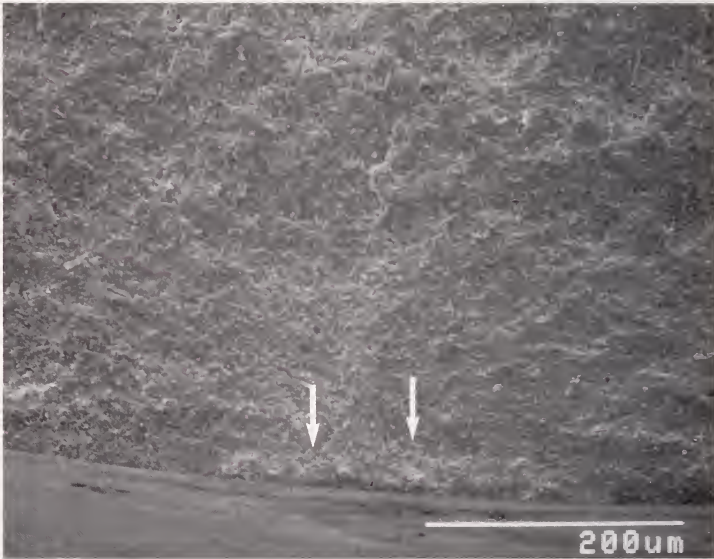
Figure 7.32 Grinding cracks in transversely ground rods that show evidence of stable crack extension (arrows) in a silicon nitride with rising R-curve behavior. (a) 657 MPa and (b) 641 MPa. (Ref. 71)
