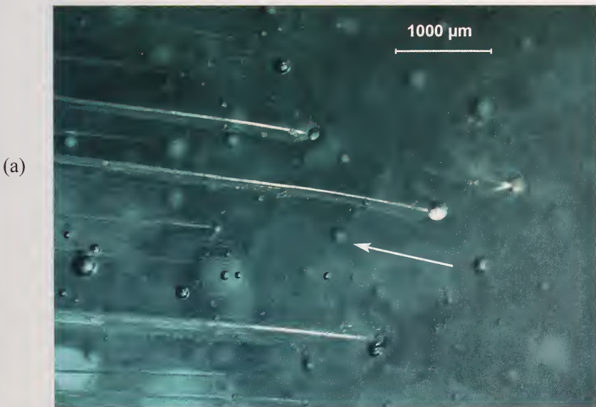
Figure 5.21 Wake hackle, the fractographers "weather vane" for crack propagation. (a) shows wake hackle from bubbles in glass. The crack was running in the direction of the arrow. Many bubbles are beneath the surface in this view.
