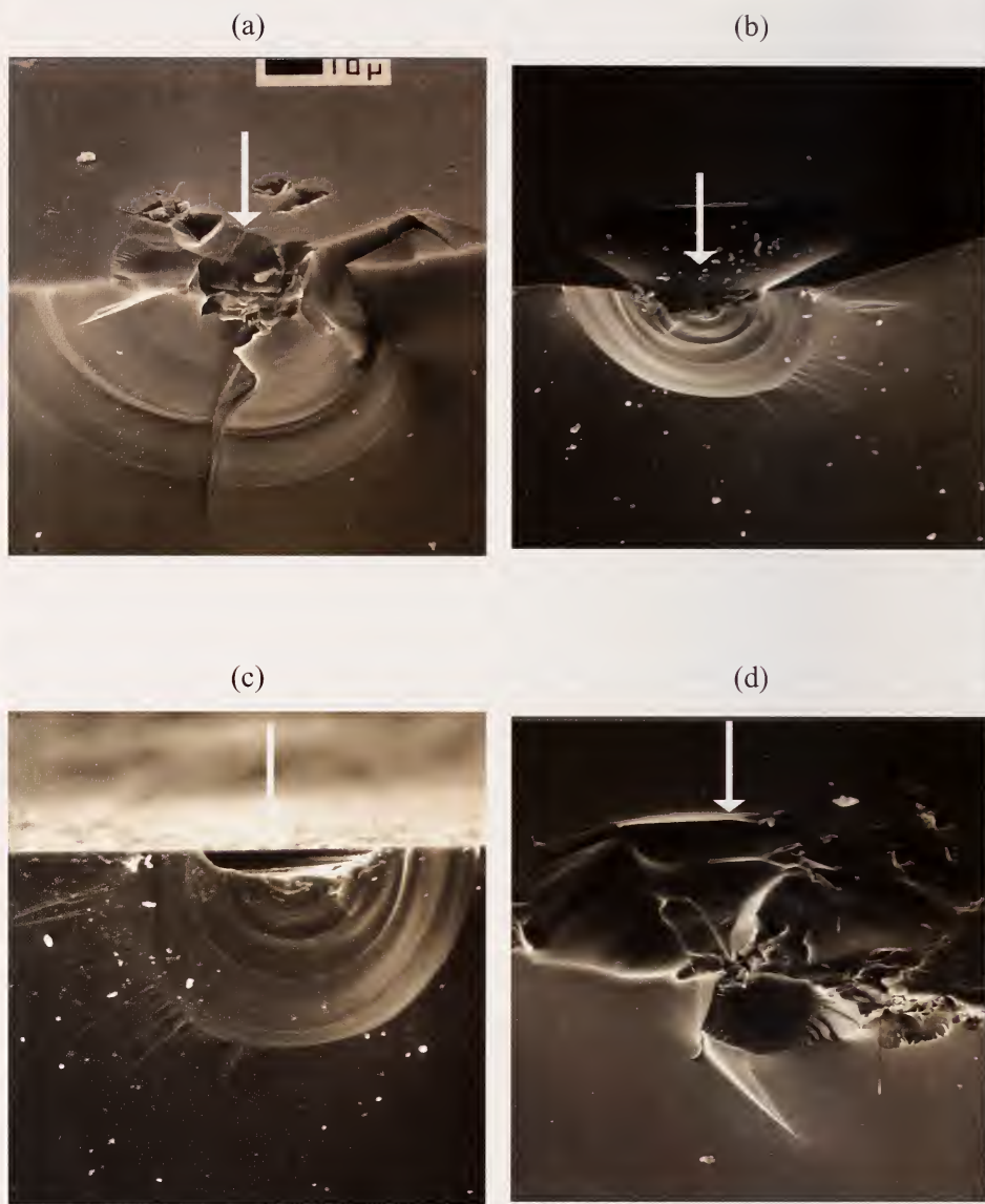
Figure 6.18. Examples of sharp particle impact origins. (a) - (d) show origins in glass. The direction of impact is shown by the arrows. All of the impacts have created penetrating median – radial cracks. (b) and (d) have pronounced lateral cracks as well. In each case the impact site has been pulverized or crushed, unlike blunt impact sites. (all Courtesy J. Varner).
