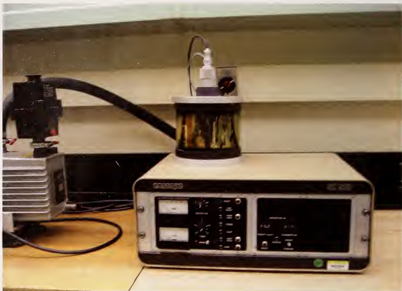
Figure 3.36. A gold sputter coater used to apply conductive coating.
