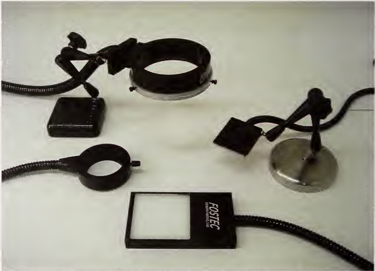
Figure 3.13. Illumination sources for use with a stereomicroscope. Clockwise from the middle left: a ring light intended to be clamped to the objective lens, a ring dark light illuminator on an adjustable stand, a line light source on a stand, and a transmitted light platform.
