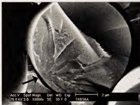
Figure 9.4. Fracture surface of an E-glass fiber reinforced epoxy matrix one-dimensional composite. The arrow marks the origin in (b). (courtesy of S. Scherrer)
