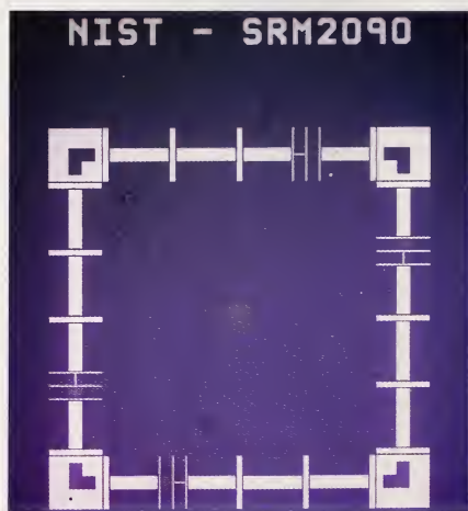
Figure 3.43. A NIST Standard Reference Material SEM length calibration standard. Finely spaced reference lines are located at intervals along the sides of the box on the right close up view.
