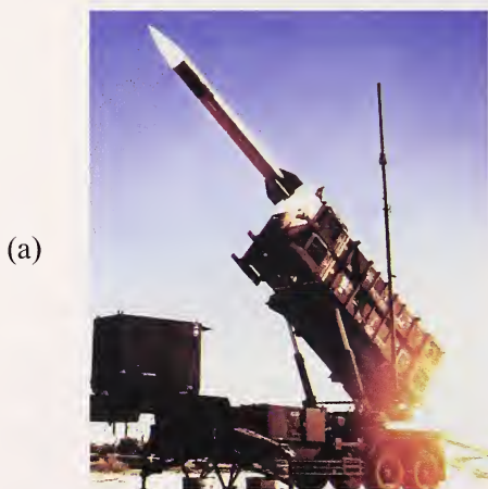
Figure 10.21. U. S. Army first generation Patriot air defense missile. The radome was 1.1 m tall with a 40 cm diameter. (a) courtesy U. S. Army. (b) courtesy Raytheon.
