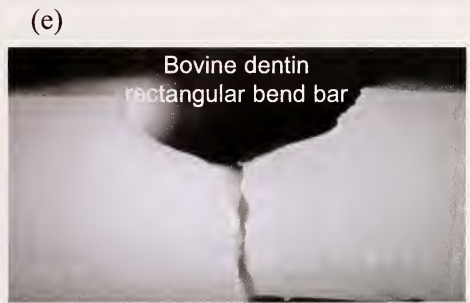
Figure 4.10 Compression or cantilever curls are a telltale feature of flexural fractures. In each case the tension surface is on the bottom and the compression surface is on top. (b) - (e) show side views of four-point flexure specimens.
