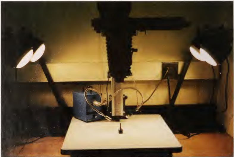
Figure 3.9. Camera stand with built-in lamps. A fiber optic light source is also on the platform to furnish vicinal (described below) and highlight illumination.
