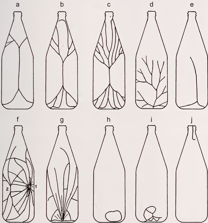
Figure 4.22 Bottle fracture patterns. (a-c) sidewall fractures due to internal pressure at progressively greater pressures; (d) internal pressure fracture starting from the base; (e) is a thermal fracture from sudden cooling of the base; (f) is an impact fracture on the right side (labeled 1) with a hinge fracture on the side (labeled 2); (g-i) show water hammer fractures and (j) shows a fracture from diametral rim clamping.
