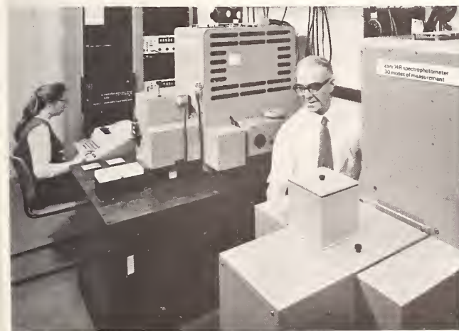
PLATE 5. View of the NPL on-line spectrophotometry data-system, showing the dedicated Micro 16P computer with 16K of core to which the two spectrophotometers shown in the foreground are interfaced in a time-sharing mode for independent operation and processing.
