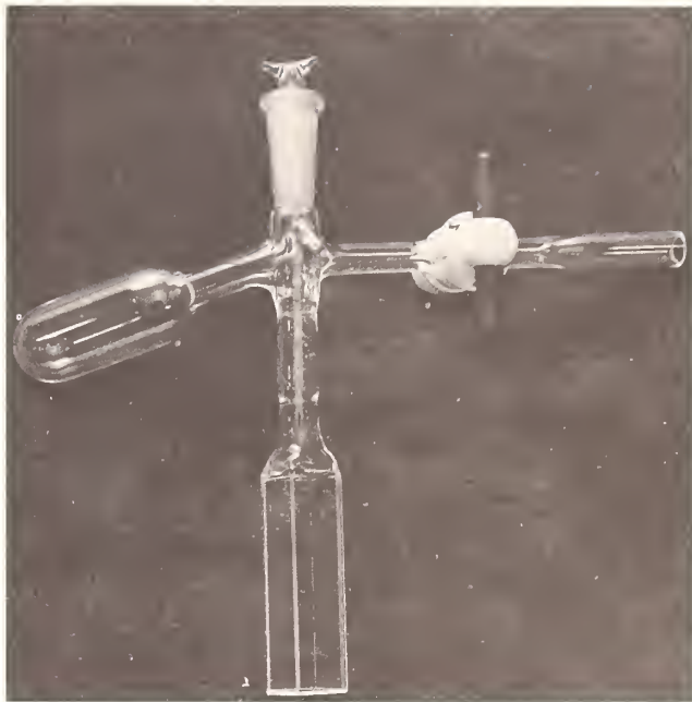
FIGURE 13. Schlenk type [76] spectrofluorimeter cell used with nitrogen manifold for degassing solutions.
