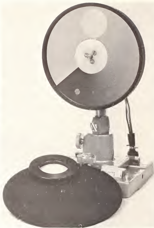
FIGURE 4. Close view of the circular, neutral wedge. The front plate which carries the fused silica lens was removed to show the fused silica disc with the evaporated metal layer.
