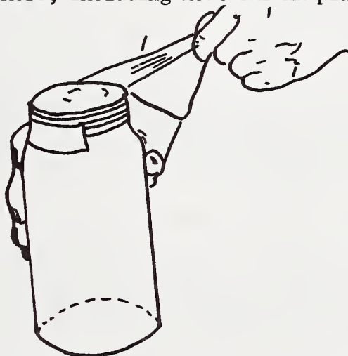
Figure 65. Use of tape as a secondary closure for glass containers.
