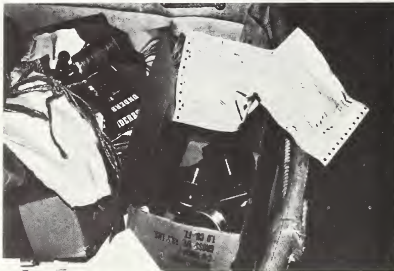
Figure 3. Inadequately packaged parcels at a Parcel Post re-wrapping station. (Some of the contents of these parcels have been lost.)
