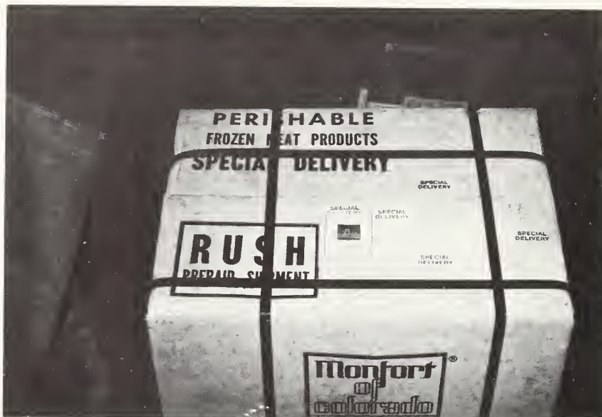
Figure 62. Appropriate use of steel strapping.
