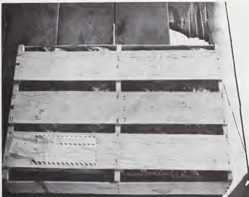
Figure 20. Wood crate, stapled and nailed. (NBS)
