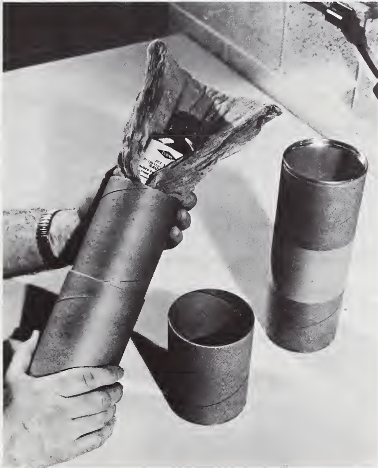
Figure 38. Cellulose wadding protecting the contents of a mailing tube.
