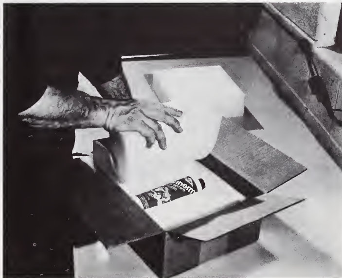
Figure 25. Corner and edge protectors of polyethylene foam.
