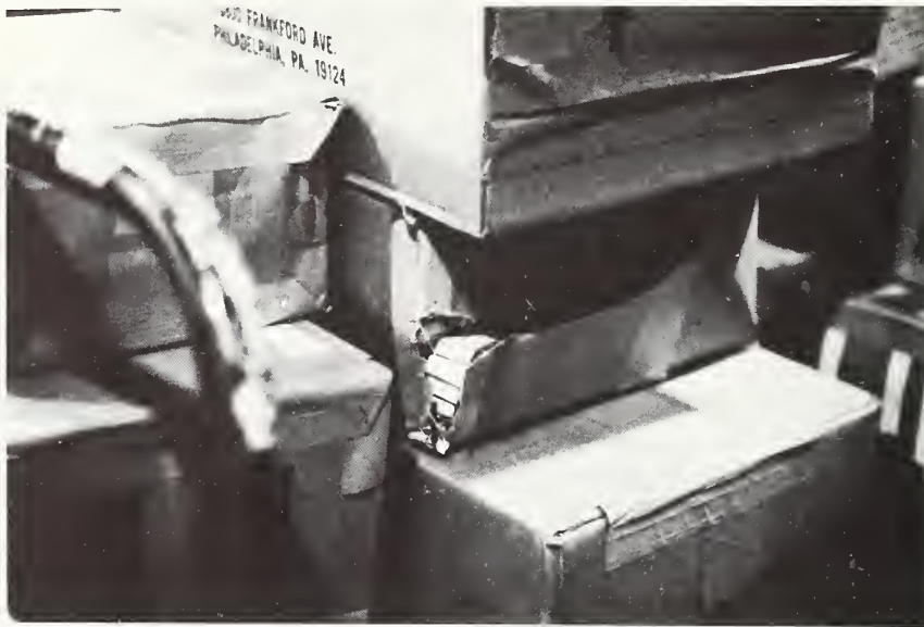
Figure 12. Damaged parcel containing documents NOT internally bound.
