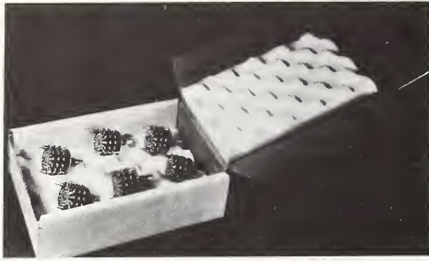
Figure 27. Protection of electronic components with expanded polyethylene.
