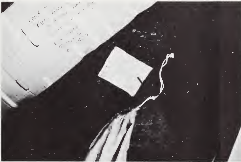
Figure 68. Tag inadequately secured with yarn.
