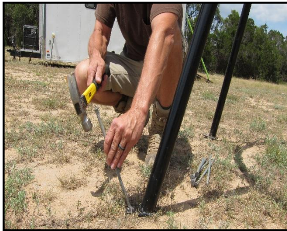
Figure 42: Once the catapult is adjusted and sitting in a level position, anchor the catapult to the ground using large spikes. Drive the spikes at an angle into the ground.
