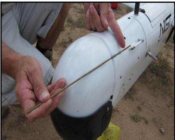
Figure 77: Slide the pitot tube into the mounting point on the airframe.
