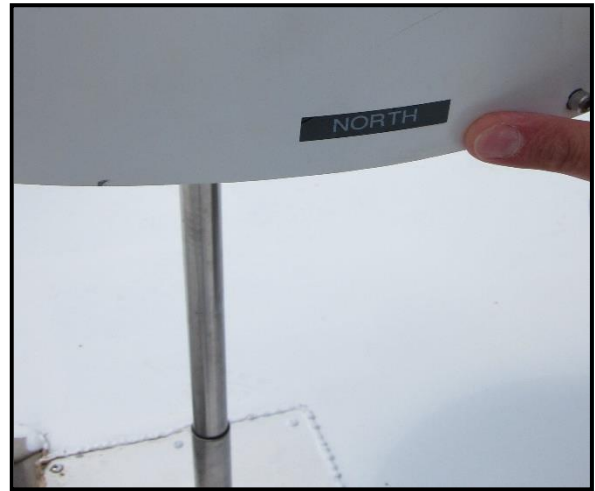
Figure 11: When placing the radome antennas insure that the NORTH label, on each radome, is facing true north.
