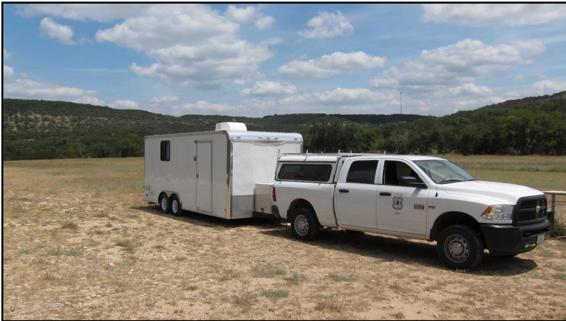
Figure 1: When placing the trailer for field operations place the door of the trailer away from the operational area and the window (above the command and control workstation) to the catapult staging, launch and recovery area.
