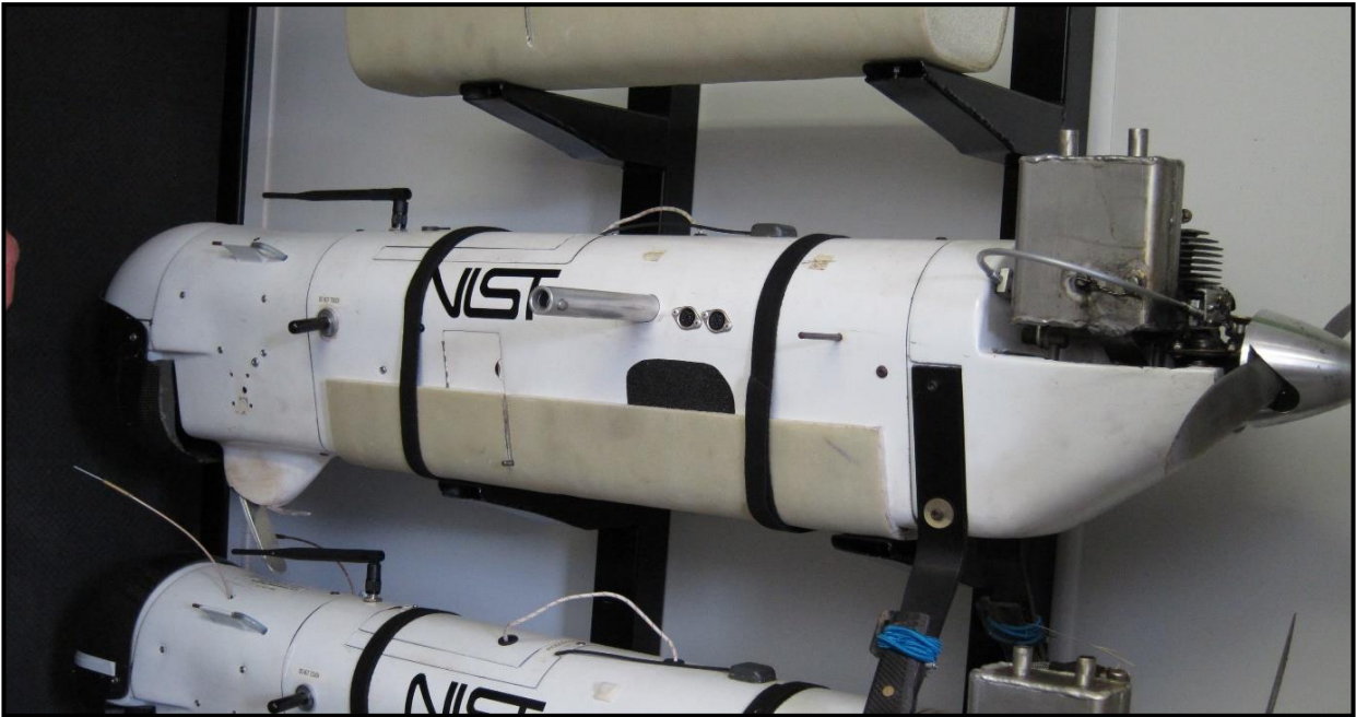
Figure 49: All airframes are secured in rear interior of trailer. Each is secured into the storage rack with Velcro straps. A retaining pin sits in a groove on each storage shelf. Use caution when removing airframe to insure no damage to airframe structure.
