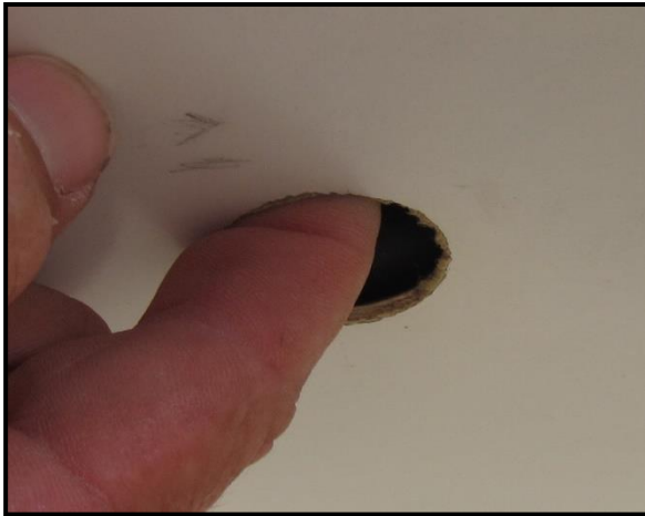
Figure 58: After wing is slid onto the mounting guide, place finger into hole to confirm mounting pin is secured.
