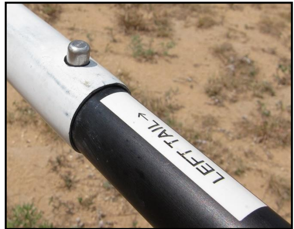
Figure 66: Visual confirmation of the securing pin deployment, on RIGHT tail boom to cathedral tail mount.
