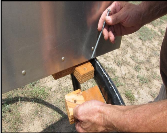
Figure 43: After the catapult, inside its transport housing, is in place; thread the support bracket carriage.
