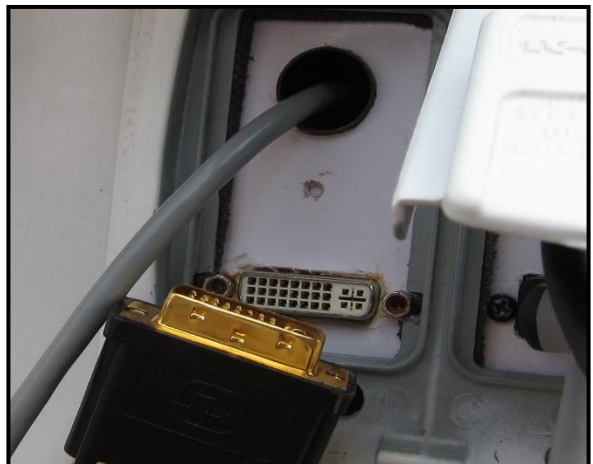
Figure 35: Locate the DVI-D bulkhead port on the trailer exterior. Connect the exterior monitor cable.
