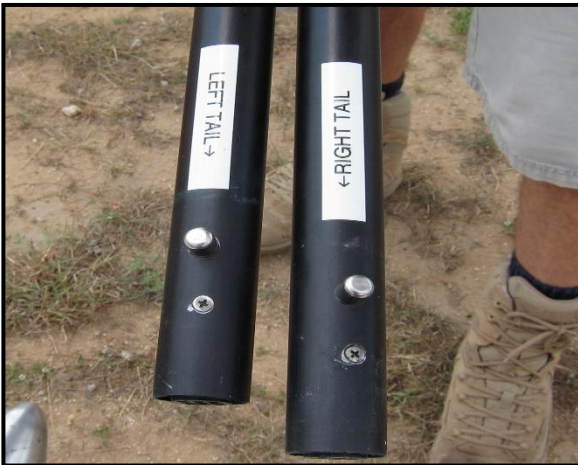
Figure 59: Identify not only the airframe identifier, but also the RIGHT and LEFT identifier before tail assembly.
