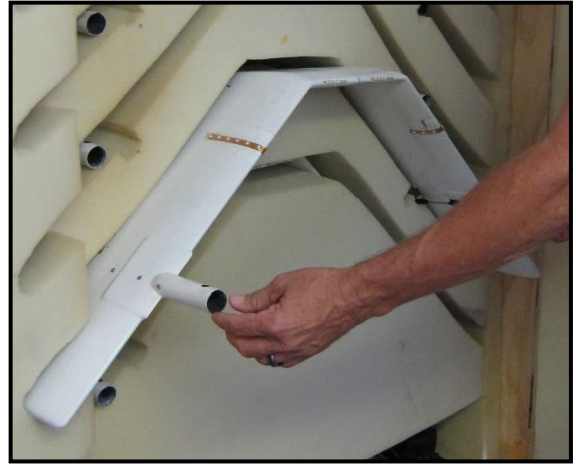
Figure 53: Select the proper cathedral tail section, by identifier number, from the storage cabinet.
