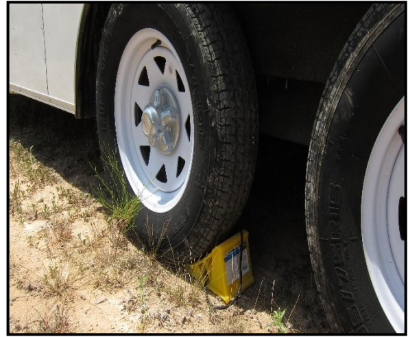
Figure 3: Before lowering the trailer support jack (front tongue on trailer) place the tire chocks securely under wheels, one on each side of trailer. Then lower the support jack.
