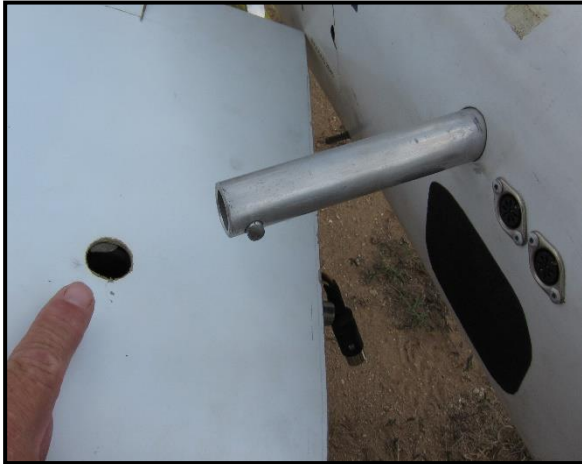
Figure 56: Identify the mounting pin access hole, on the bottom aspect of the wing.
