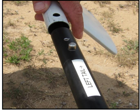
Figure 64: Follow the same procedure for placement of the securing pin as the wing set and tail boom to wing set.
