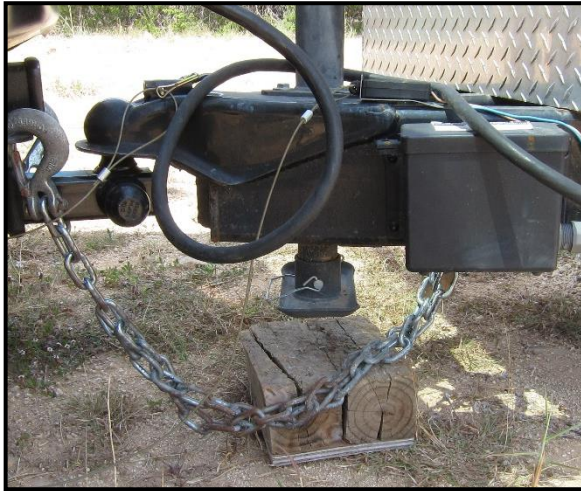
Figure 2: The trailer must be completely disconnected from the tow vehicle before lowering the support jack. These same connections must be in place before towing trailer from operation site.
