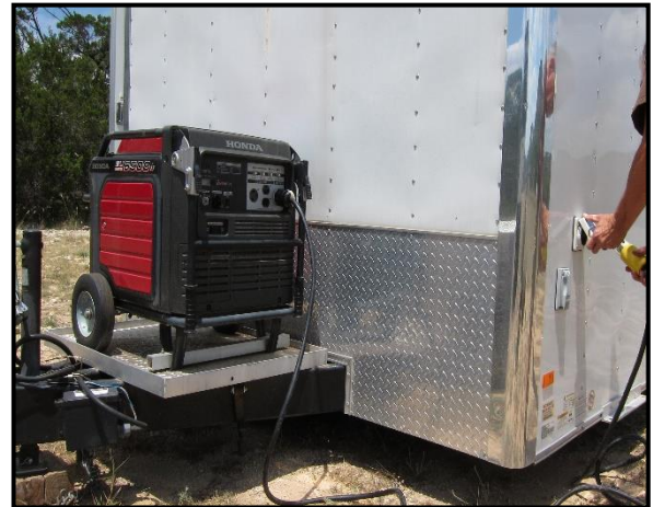
Figure 7: Plug the generator power cable in to the generator and the trailer.
