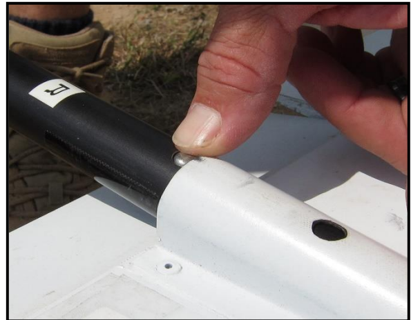
Figure 62: Depress the securing pin while inserting the tail boom section in to the mounting guide on the wing.
