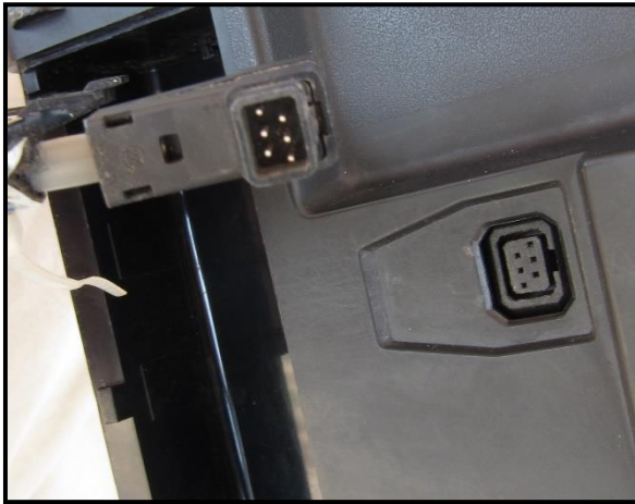
Figure 32: Locate the PIC controller GCS cable and match the pin placement.
