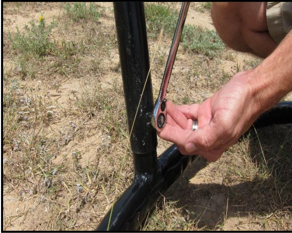
Figure 40: After all legs are in place, tighten all attachment bolts with a box or open end wrench.
