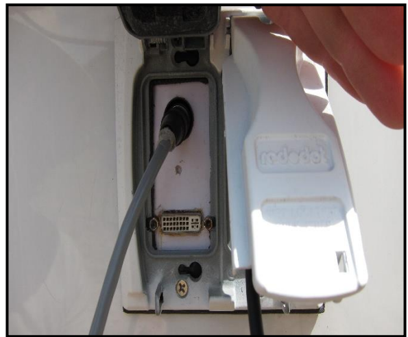
Figure 31: Insure the cable is inserted with enough slack to reach the GCS unit inside the trailer. Use caution when closing the bulkhead cover to prevent any damage to the cable.
