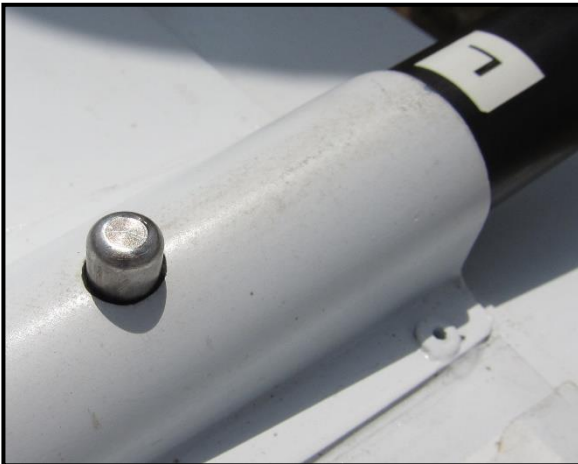
Figure 61: When the tail boom is secured an audible click will be heard. The deployment of the securing pin can also be visible.
