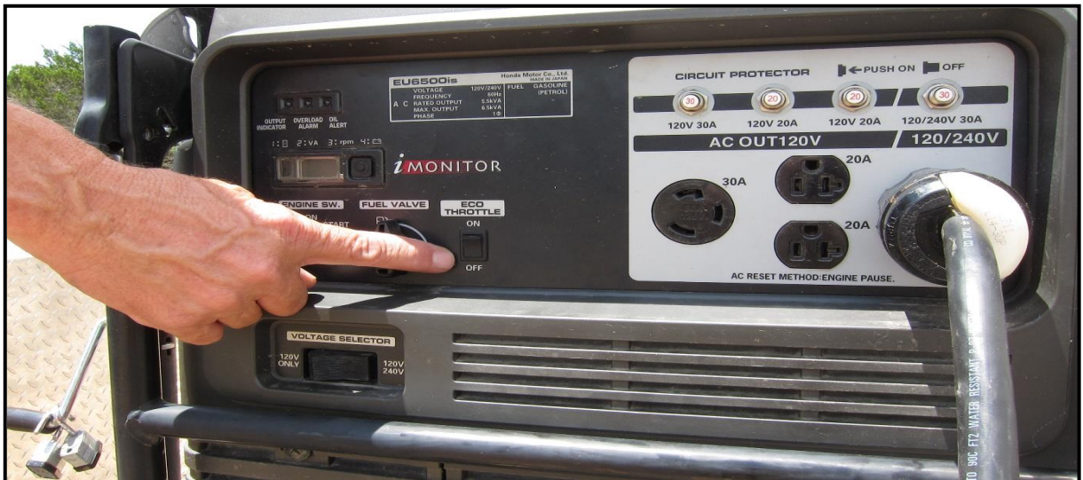
Figure 8: Check that the generator is switched into the 'OFF' position in the ECO Throttle mode before starting. Allow the generator to run in the 'OFF' ECO mode for several minutes before switching into ECO mode before continuing trailer power up procedures.
