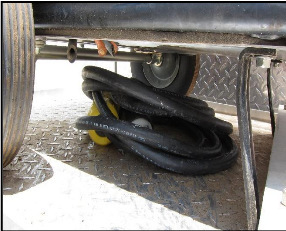
Figure 6: Once the generator cover is removed, locate the generator power cord stored beneath the generator.
