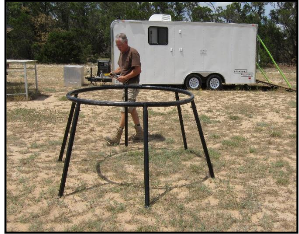
Figure 41: After all legs are secured, rotate the catapult ring to its upright position.
