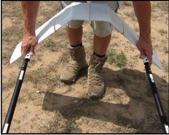
Figure 63: Following the secure placement of the tail booms, slide the cathedral tail onto the booms.
