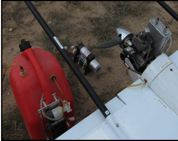
Figure 85: Once a secure connection is confirmed, commence fueling procedures.
