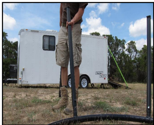
Figure 39: To assemble the legs to the main catapult place the ring upside down and insert each leg. Loosely tighten the attachment bolts on each leg by hand.
