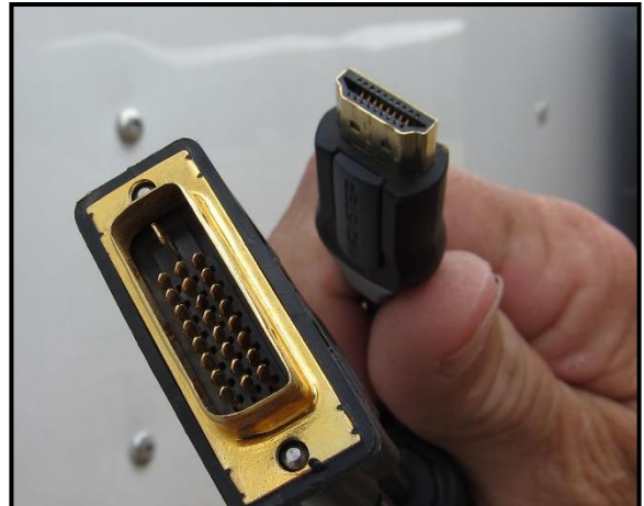
Figure 37: The DVI-D and HDMI cable will be required along with monitor power cable for external mounting and proper operation of external monitor.
