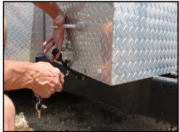
Figure 5: After the trailer is secured, the generator cover can be unlocked and the rubber secure straps unhooked.
