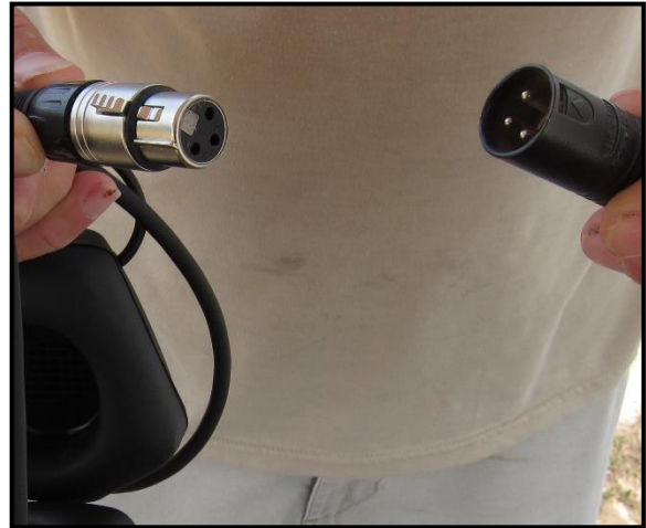
Figure 29: Attach the male XLR from the headset to the female XLR extension that is connected into the bulkhead XLR bulkhead port.
