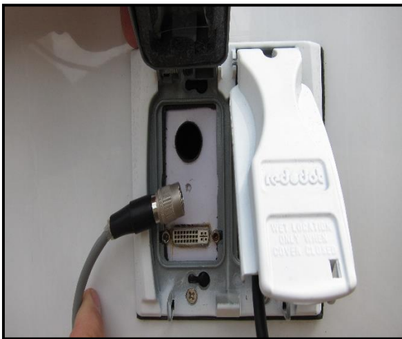
Figure 30: Insert the GCS connection side of the PIC transmitter control cable through the open port in the trailer bulkhead.
