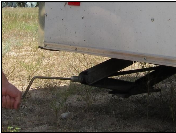
Figure 4: Following the placement of the tire chocks and lowering the support jack (front tongue on trailer), the rear support jacks can be lowered.
