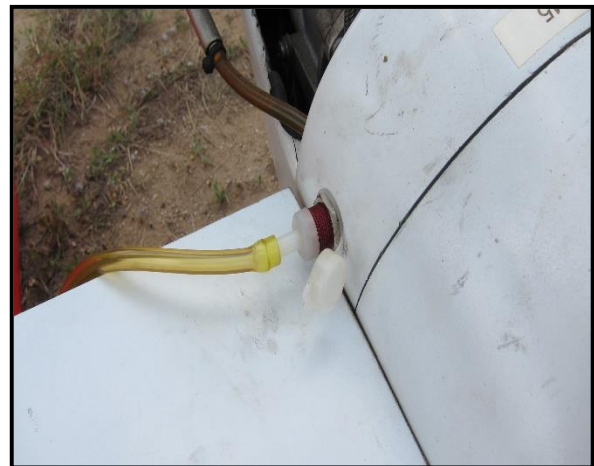
Figure 84: Attach the fueling line from the fuel canister to the fueling port on the airframe.
