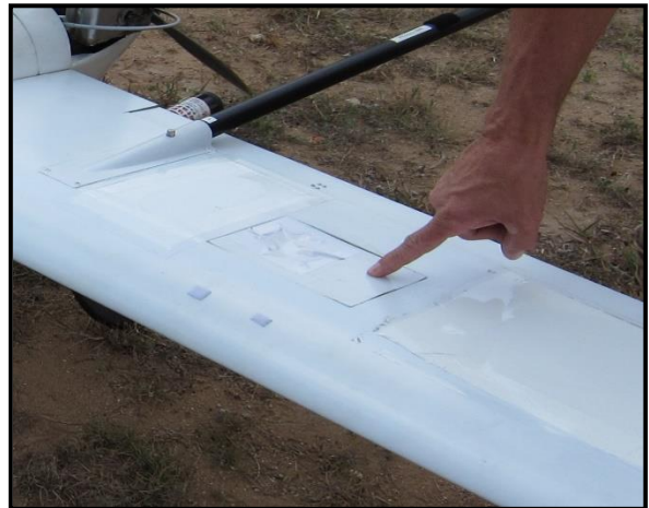
Figure 82: After camera system is secured into the bay, replace the cover. Insure cover is secure.
