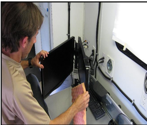
Figure 17: Remove transport padding and open PAC monitor mount
