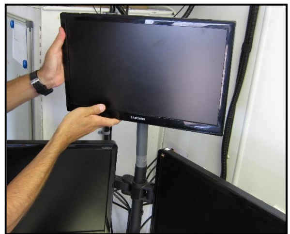
Figure 18: Secure the external field view monitor into the open tube of the PAC monitor mount.
