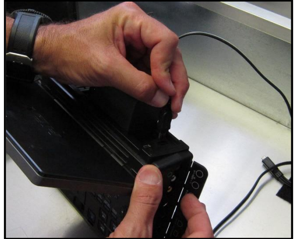
Figure 24: Connect the power cable, to both HDV decks. Power connection is on rear of the deck.
