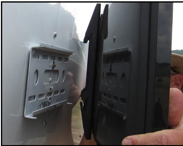
Figure 34: Locate the exterior monitor mount on the exterior trailer. Align mounting brackets and confirm secure placement of monitor. It is advisable to attach the DVI-D, HDMI and monitor power cable before mounting.
