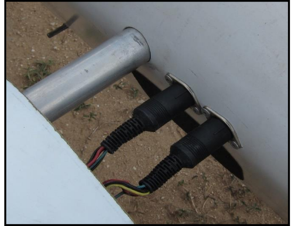
Figure 57: Connect both wing control cables to airframe. Confirm secure connection before continuing with wing assembly.
