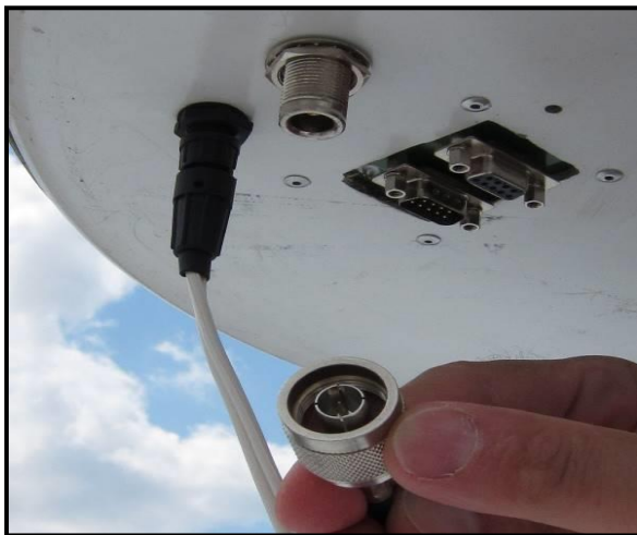
Figure 14: Attach the N-type connector, video line, to each random unit.
