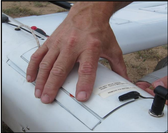
Figure 71: Re-insert the parachute by mechanism into the bay, using caution to avoid pinching or obstructing any of the parachute mechanism wires or cord.
