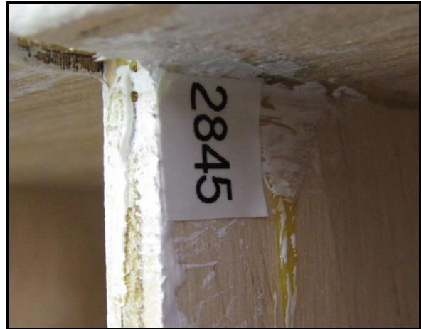
Figure 51: Insure the proper wing-set is used based on airframe selected. Match and confirm the identifier number.
