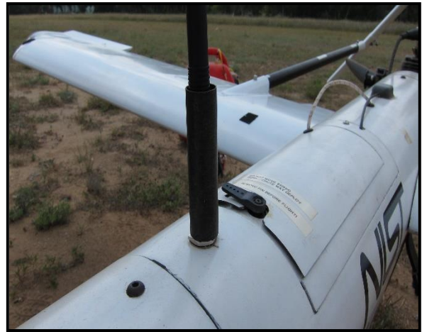
Figure 76: Confirm collar is sitting against the mounting base of the antenna and that the telemetry antenna is in an upright position.
