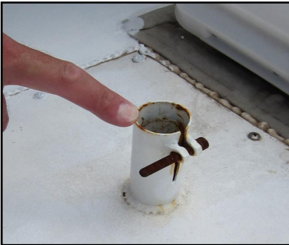
Figure 10: Locate the attachment point for the video tracking radome antennas on the trailer roof. NOTE: There are two different size attachment points (the mounting poles for the radome's are different diameters).
