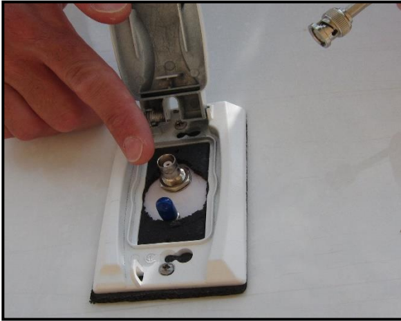
Figure 9: Locate the bulk head BNC connector on the exterior trailer to connect the external telemetry antenna cable.
