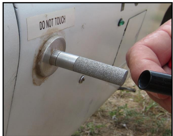
Figure 74: Gently remove the plastic sensor cover from the sensor. Use caution to not dislodge or rotate the sensor during removal of the cover.
