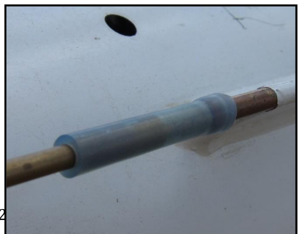
Figure 74: Once the tube is inserted, slide the rubber sheath over the mounting point and confirm the tube is secure.
