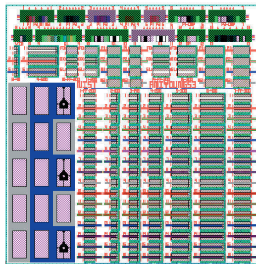
Figure 10. Test chip design fabricated on the AMI 1.5 \mu\text{m} CMOS process.
