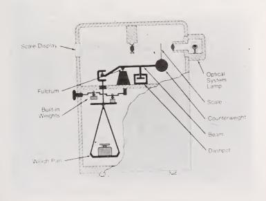
Figure 2 Laboratory Balance
