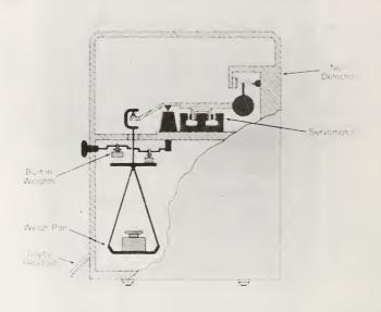
Figure 3 Balance with Servo-Motor
