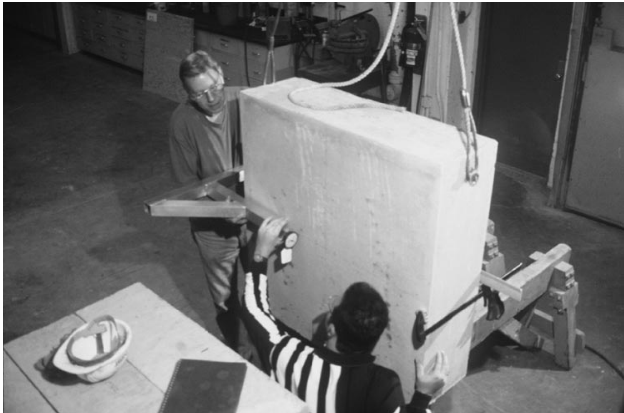
Figure 4.5: Measuring thickness variations for a nominal 305 mm thick concrete specimen.
