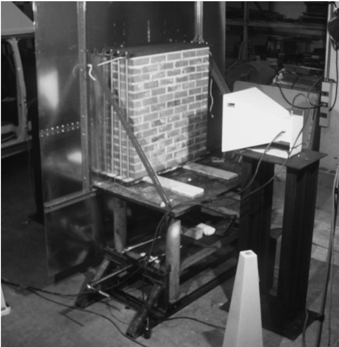
Figure 4.1: Test setup for specimen B3L (three-wythe deep brick wall) for frequency response determination from 0.5 to 2.0 GHz. See Figures 4.1a and 4.1b.
