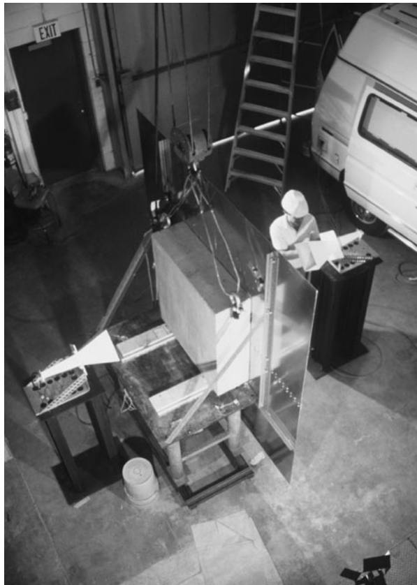
Figure 4.4: Test setup for specimen C112H (305 mm thick plain concrete wall) for frequency response determination from 3.0 to 8.0 GHz. See Figures 4.4c and 4.4d.
