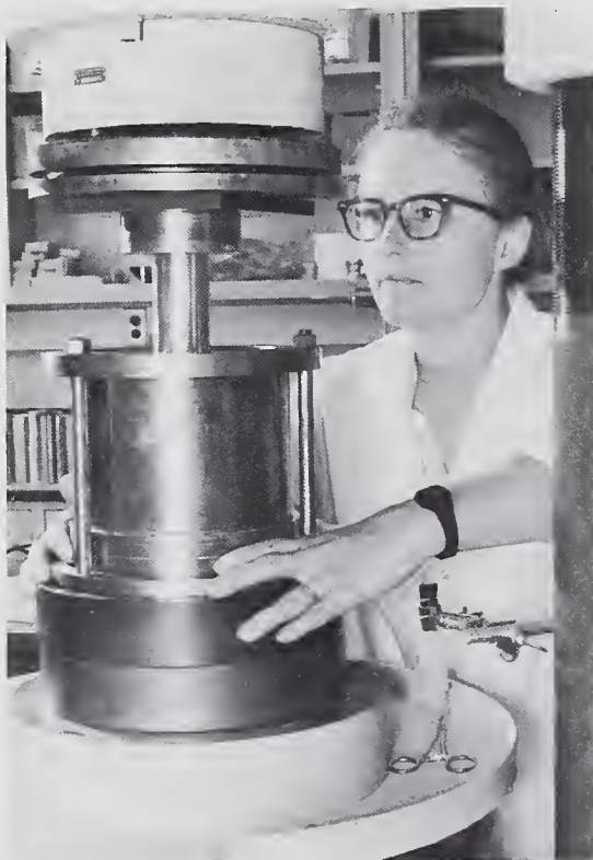
Dr. Leslie Struble uses a cylinder and piston device to study the causes of concrete failure.
