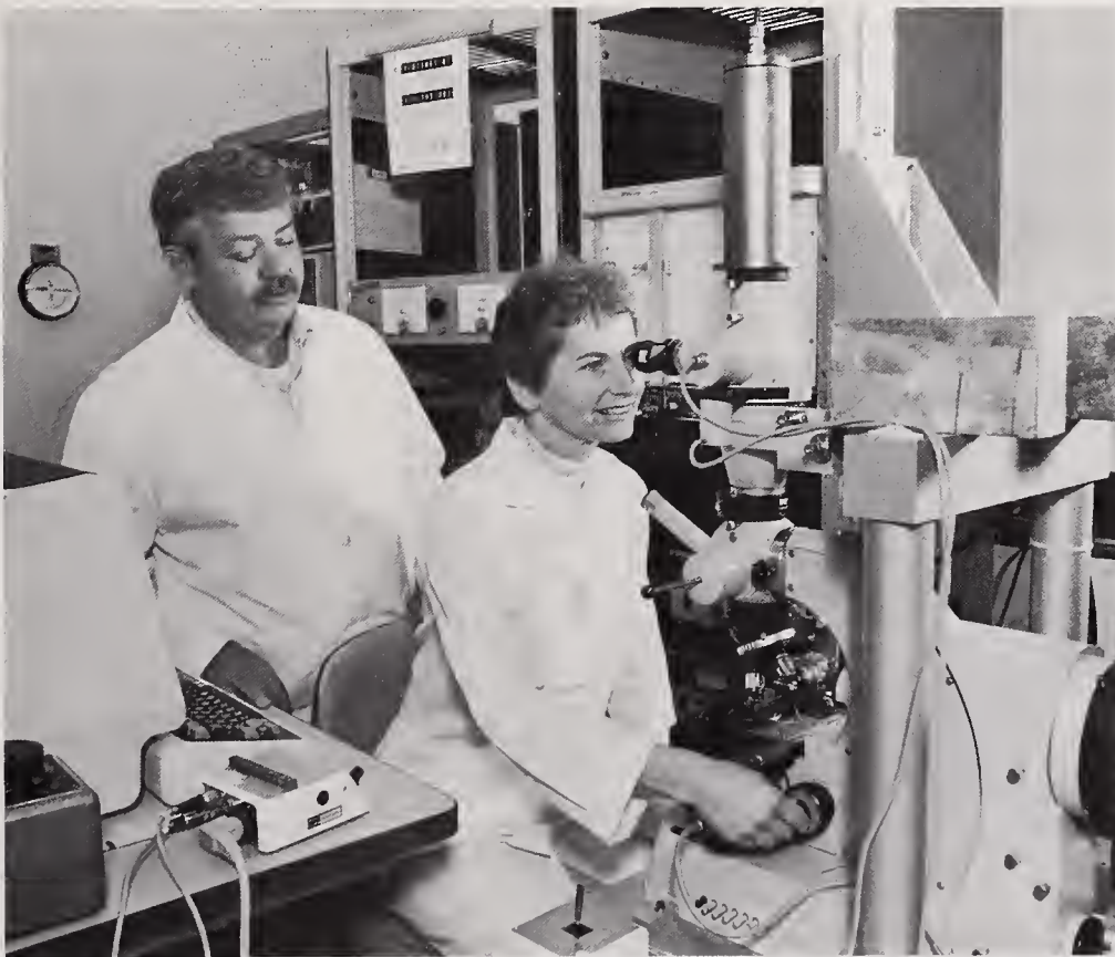
NBS scientists Carol Vezzetti and Sam Jones use a modified optical microscope linked to a data-collection computer to calibrate NBS photomask SRM's. It takes up to a week to calibrate a single photomask—an automated system under development will cut that down to a day.
