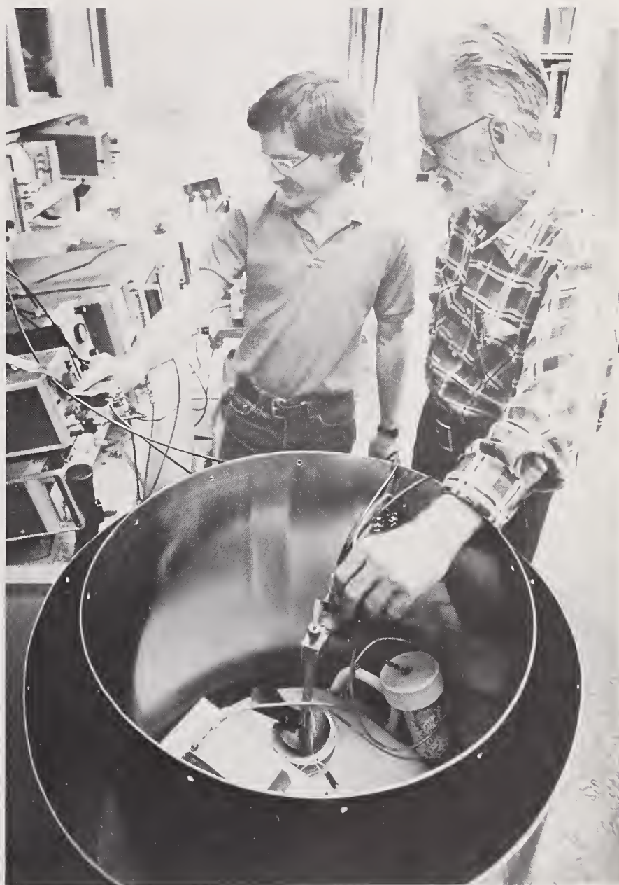
Electronics engineer James Beall (left) and physicist Dr. James Zimmerman adjust apparatus used with the high-temperature SQUID they developed and built. This SQUID may be the first practical superconducting device to operate in liquid nitrogen.
