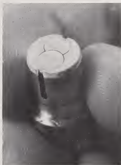
The two discs at the top of this sensor plug are part of a thin-film thermocouple system that will accurately measure the internal temperature of a diesel engine.
