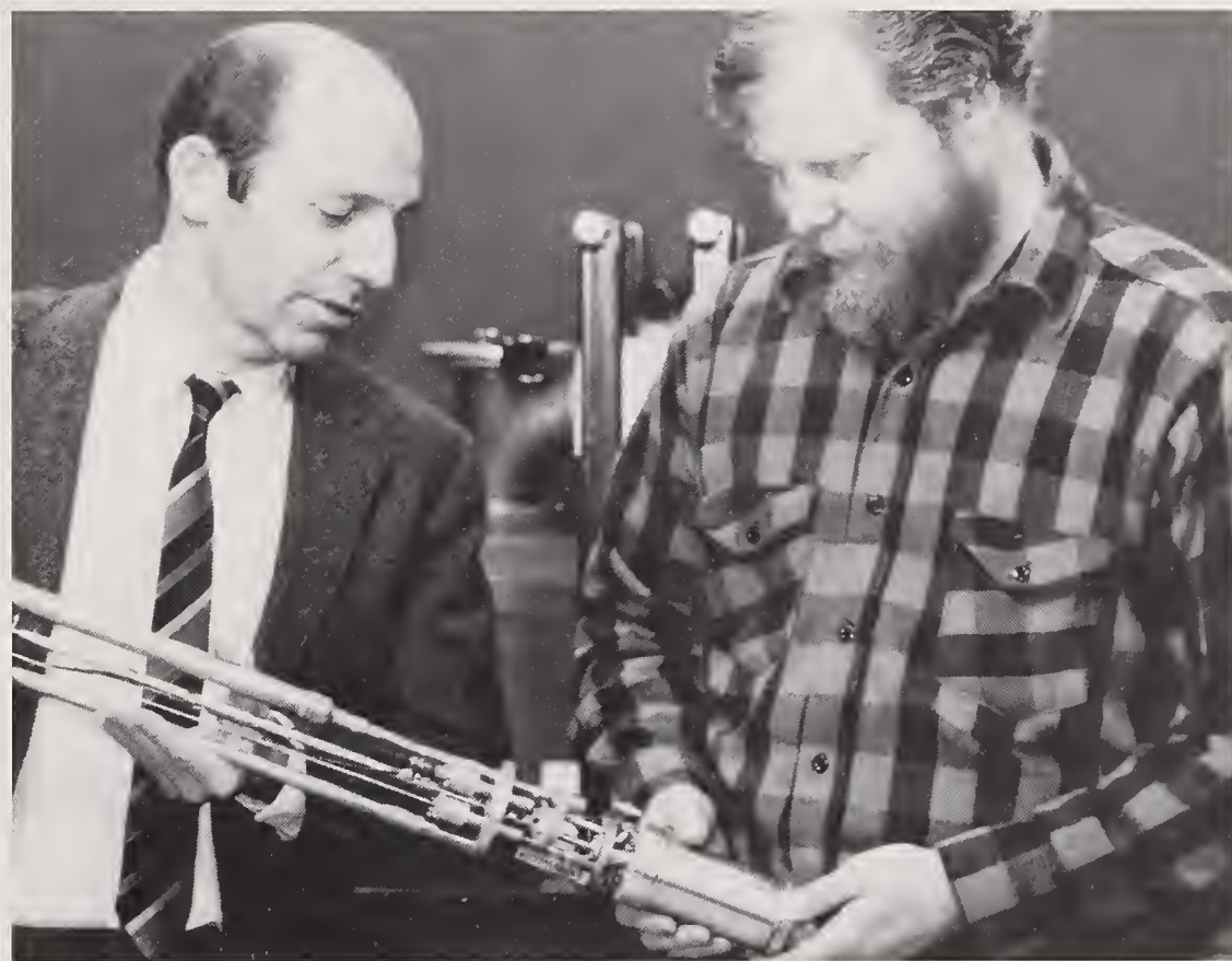
Drs. Alan Clark (left) and John Moreland use a break junction apparatus devised by Moreland to make electron tunneling measurements on the high-temperature superconductors. These measurements will help explain why the materials become superconductors at high temperatures.
