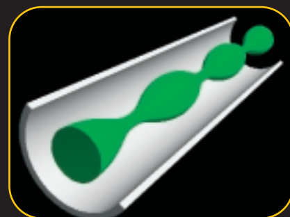
Lattice Boltzman simulation of the Taylor-Tomotika instability of a fluid thread confined within a tube.
