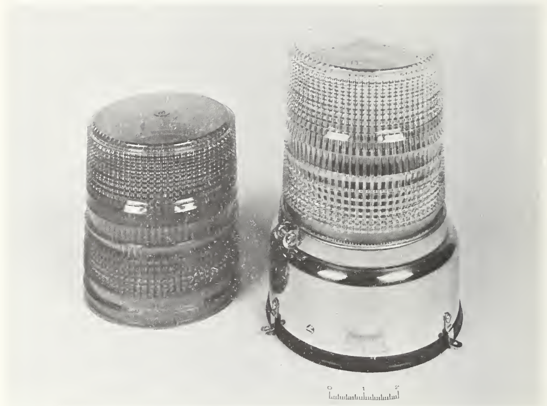
FIGURE 3.4f. Single xenon flashtube is energized through built-in, high-voltage, condenser-discharge circuitry, under base. Clear dome contains built-in Fresnel lens (horizontal ridges) that acts as a uniform, wraparound cylindrical lens, concentrating the light around the horizontal plane evenly over a full 360°. Dome also features superimposed straight vertical “ribs” that diffuse the light across the entire width of the dome. Substitutable colored dome is also shown on the left. A single, small, upright, nonreflectorized incandescent lamp is also mounted under the dome and is burned steadily to permit continuous visibility of the unit at close ranges at night.
