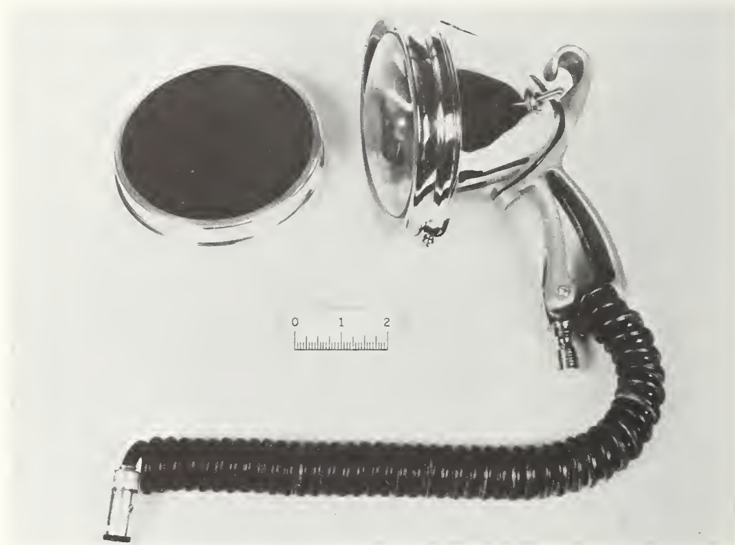
FIGURE 3.4b. Hand-held, pistol-grip, single-lamp warning spotlight. Lamp is incandescent sealed beam (PAR) type, and flashes by current interruption. Unit shown with clear front lens. Colored lens shown on the left can be snapped on over the clear lens.
