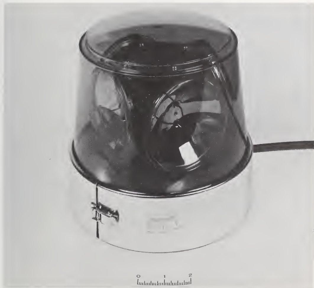
FIGURE 3.4a. Four stationary, horizontally directed sealed beam (PAR) incandescent lamps are flashed by current interruption. Unit shown has clear lamps under a colored dome.
