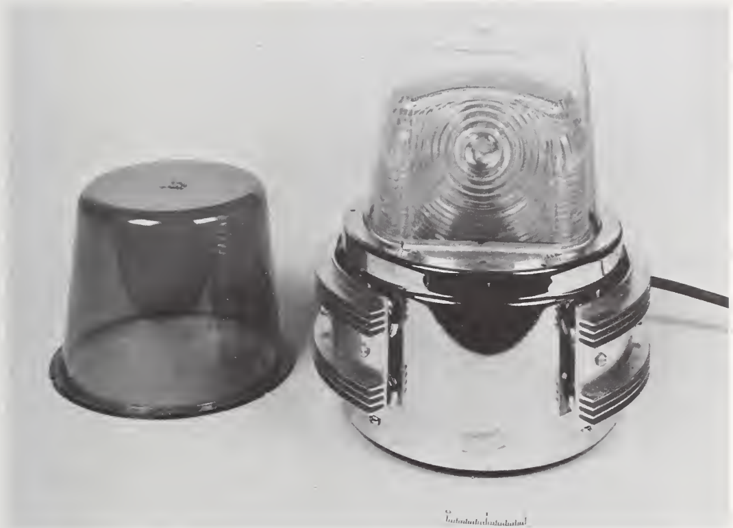
FIGURE 3.4g. Single xenon flashtube is energized through built-in, high-voltage, condenser-discharge circuitry, in base. Inner clear dome is flattened, with "hull's-eye" Fresnel lenses on both front and rear surfaces. Light emerges over 360°, but these lenses concentrate the light more strongly around the front and rear horizontal directions. The narrow side surfaces of the inner dome contain cylindrical Fresnel lenses (horizontal ridges) that concentrate the light emitted sideways around the horizontal plane. Smooth outer dome is clear, with substitutable colored outer dome also shown on the left. Also mounted under the inner dome are two small, upright, nonreflectorized incandescent lamps, one on each side. These are hurned steadily to permit continuous visibility of the unit at close ranges at night.
