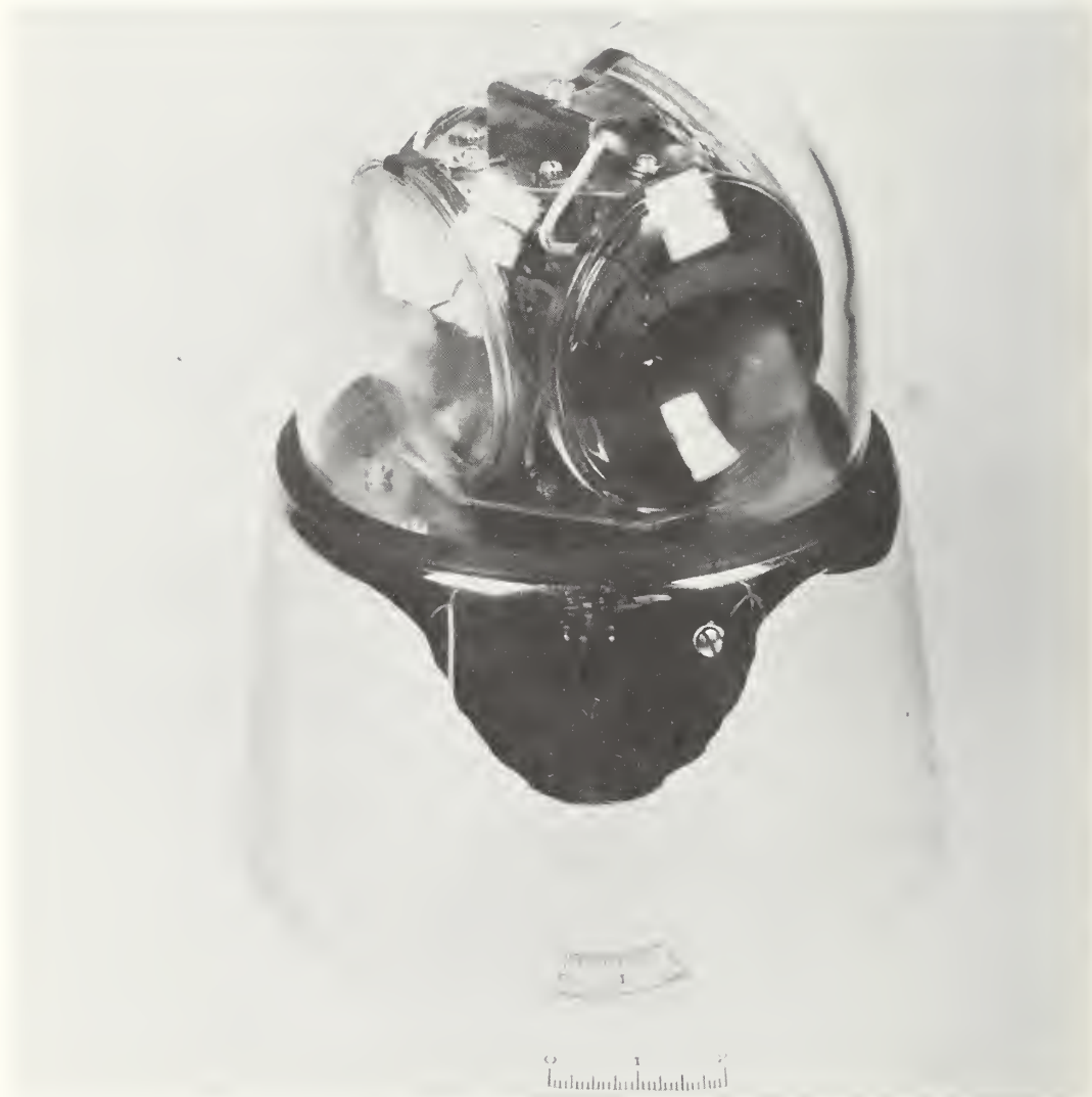
FIGURE 3.2b. Rotating base carries four sealed beam (PAR) incandescent lamps shown under a clear dome. Two opposite lamps with colored faces are directed horizontally. Two alternate lamps are clear, and one (rear right lamp) is tilted upward, the other downward.
