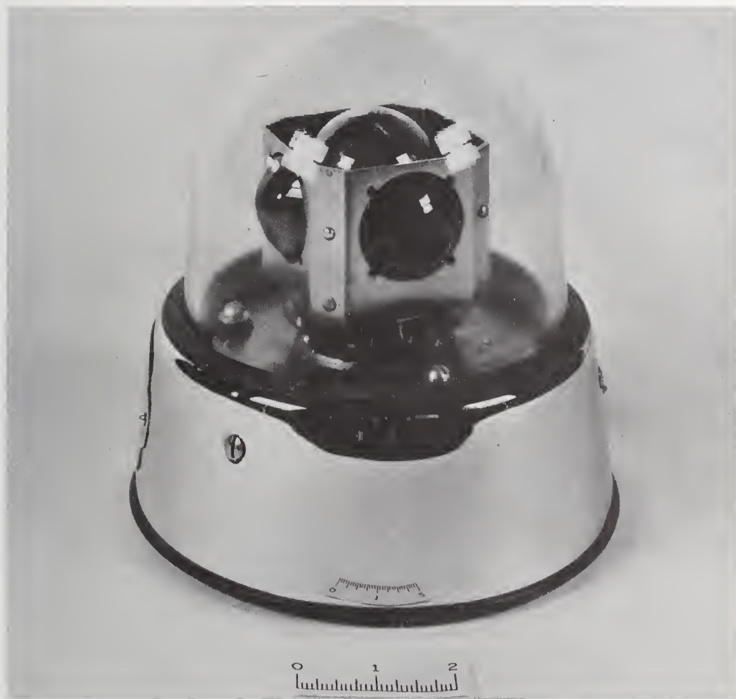
FIGURE 3.2d2. Rotating base carries four lenses around a fixed, nonreflectorized, clear incandescent lamp with its axis vertical. Unit shown has four colored lenses rotating around an upright lamp, under a clear dome.
