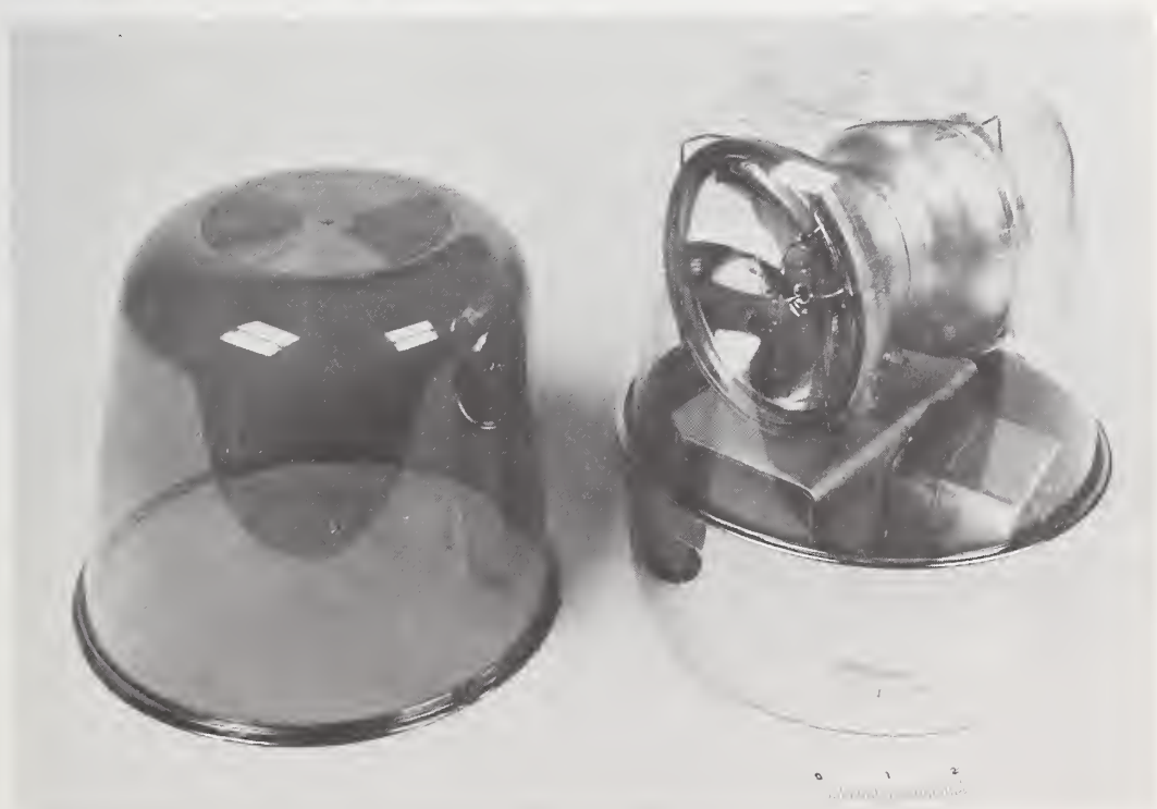
FIGURE 3.2a2. Rotating base carries three sealed beam (PAR) incandescent lamps. Unit shown has three lamps with colored dome. Substitutable colored dome also shown on the left.
