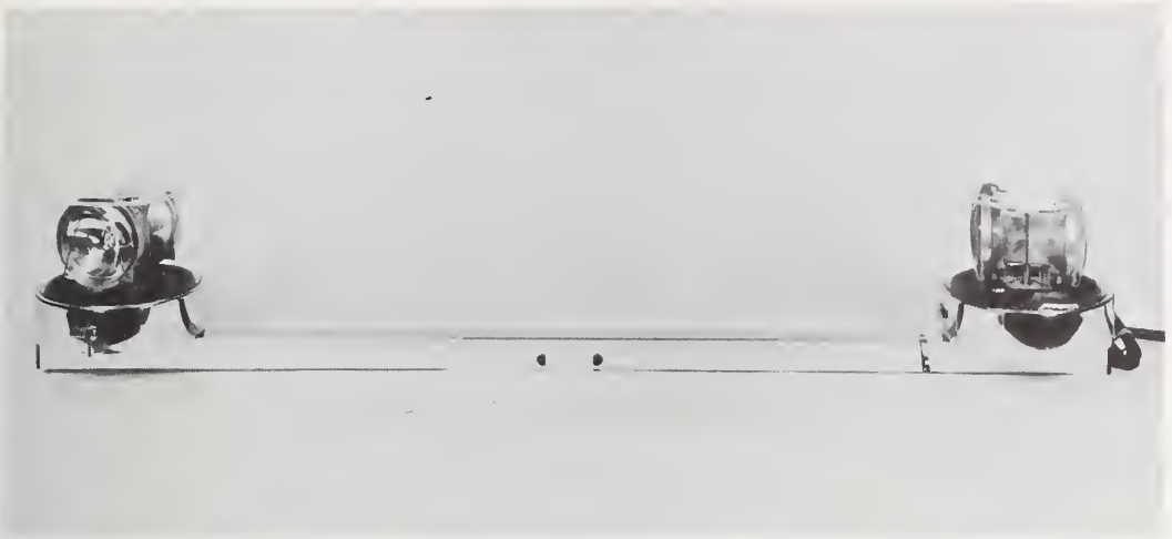
FIGURE 3.5a. Roof bar with two 2-bulb rotating incandescent units (resembling fig. 3.2a2), one at each end, rotating synchronously with 90° offset of phase (one unit oriented sideways when the other is fore-and-aft). Length of bar is 4 1/2 ft (about 1.37 m).
