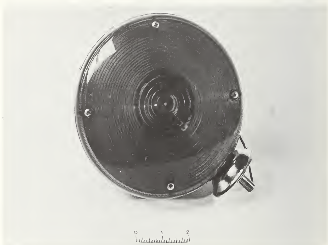
FIGURE 3.4c2. An electrically flashed incandescent unit having an optical layout similar to the light shown in the preceding figure (fig. 3.4c1), but considerably larger in diameter. Requires external flasher circuitry.
