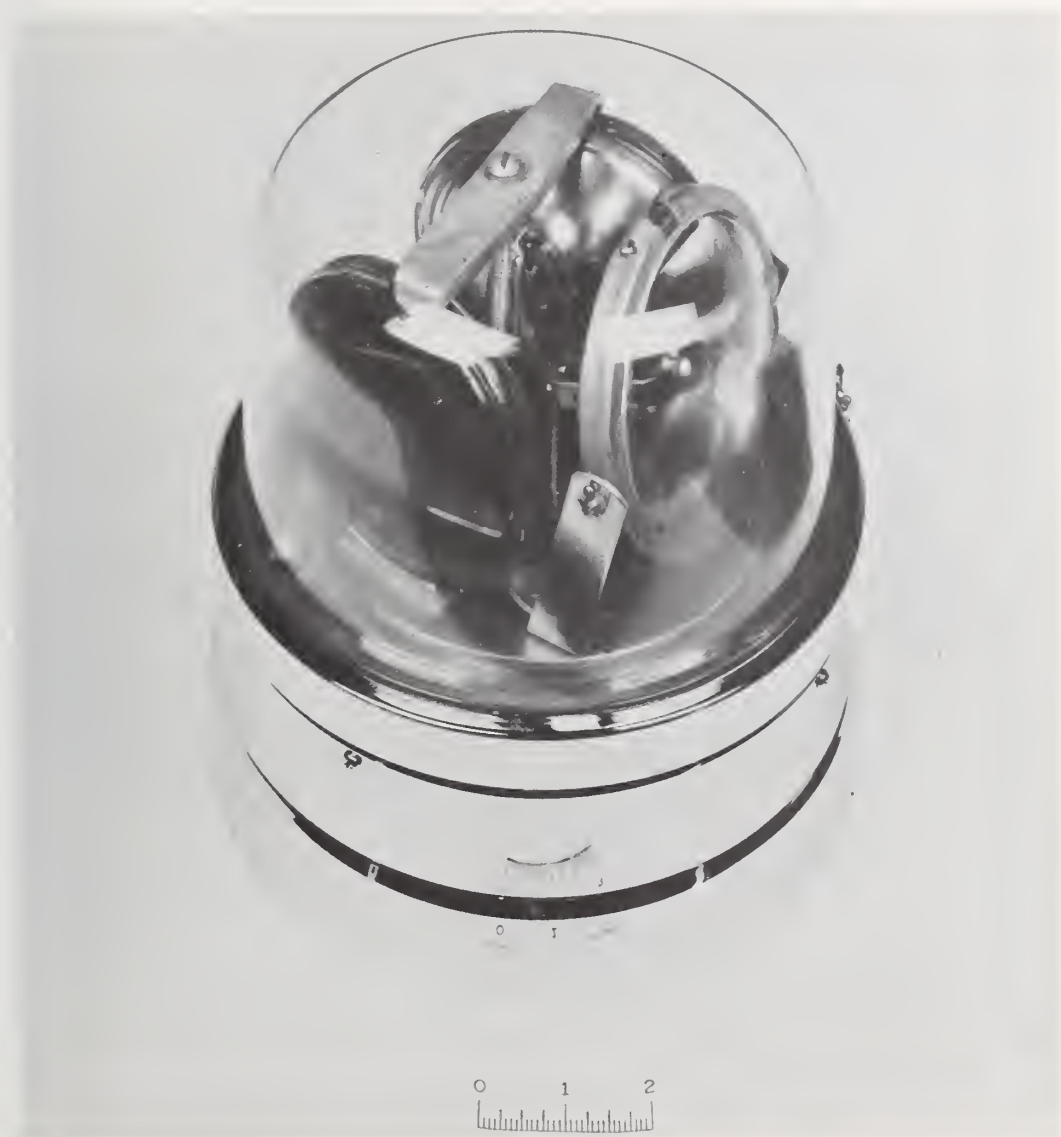
FIGURE 3.2c. Rotating base carries three sealed beam (PAR) incandescent lamps shown under a clear dome. Two lamps have colored faces and are directed horizontally. The other (right lamp) is clear and oscillates vertically as it rotates.
