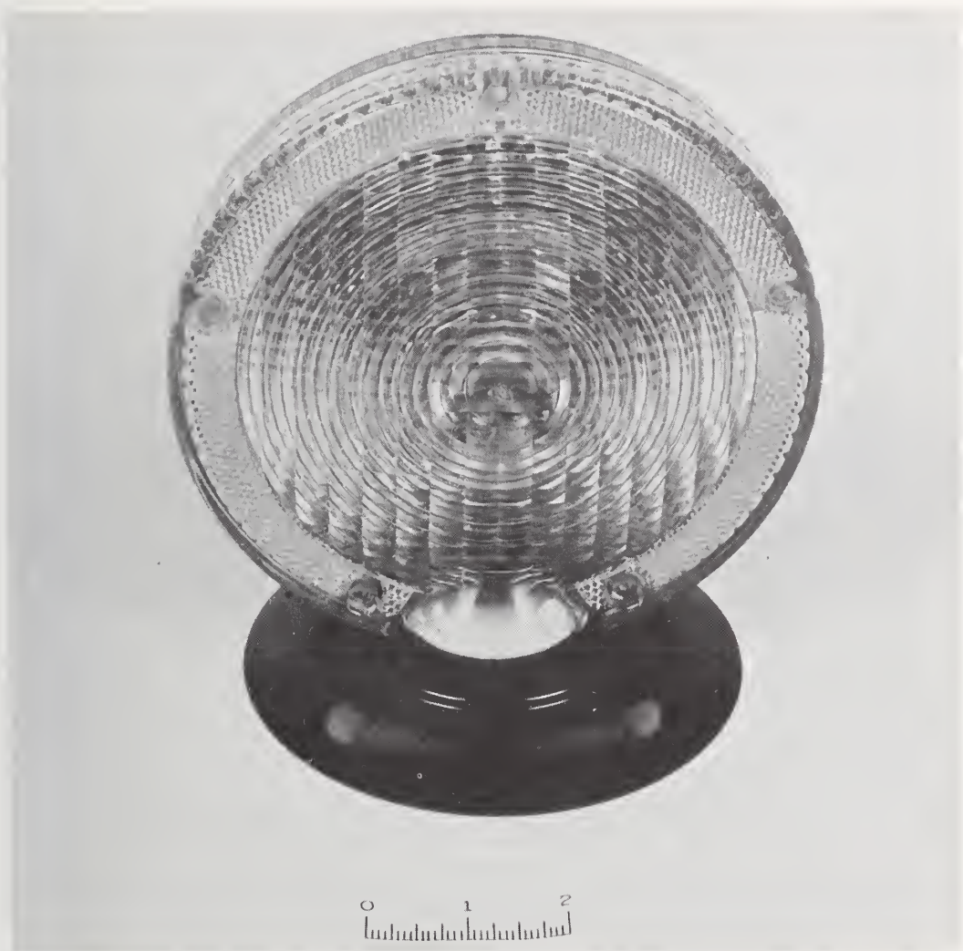
FIGURE 3.4c3. Two small, upright, nonreflectorized incandescent lamps, side by side, flash with independent phases, by current interruption. Fresnel lenses fore and aft contain not only a "bull's-eye" pattern for concentrating the beams in the forward and rearward directions, but also superimposed straight "ribs" that diffuse the light over the entire surfaces of the lenses. One lens is red and the other yellow (amber). Dual flasher circuitry is built in. Unit plugs into cigarette lighter socket, and has no attachment hardware on the base. It is intended for occasional use as a stopped-vehicle signal, and possibly also for occasional use as an internal, normally concealed, emergency-warning light.
