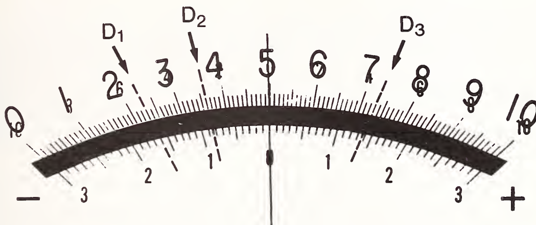
Figure 4. Typical microvoltmeter scales with three deflections marked.
