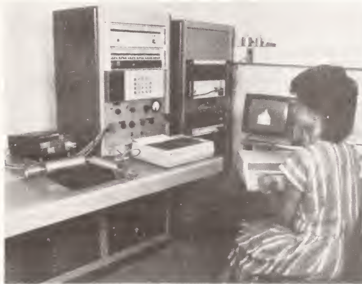
Fig. 2. Automated ac-dc difference calibration system.
