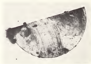
Figure 9. An autoradiogram of an irradiated Si plate (1X).
