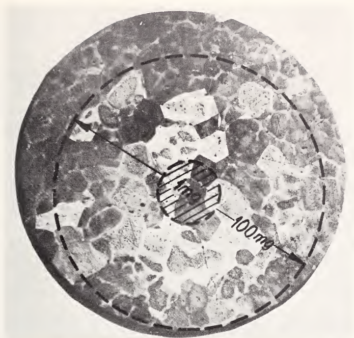
Figure 5. Structure of copper (30X) with shown diameters of 1-mg and 100-mg samples.
