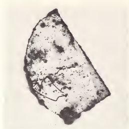
Figure 8 An autoradiogram of an irradiated Si plate (1X).
