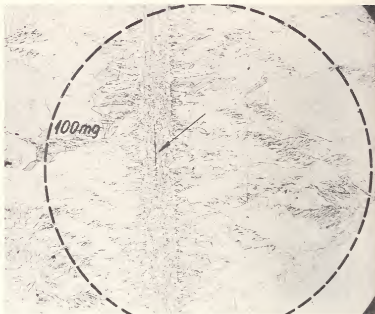
Figure 1. Structure of Armco steel with an inclusion (30X).
