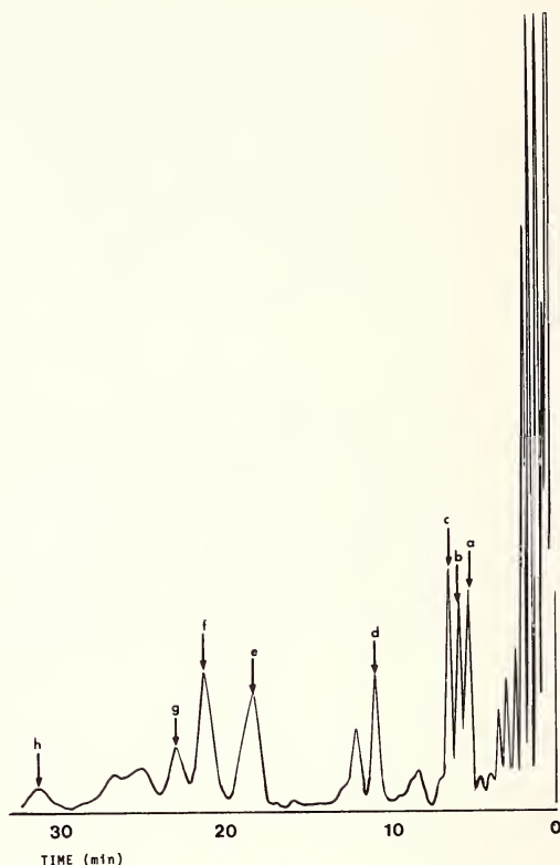
Figure 2. Chromatogram obtained from a calvados to which the following nitrosamines had been added, each at the 10 \mu\text{g/kg} level (after clean up); a) N-Nitrodimethylamine, b) N-Nitromethylethylamine, c) N-Nitrodiethylamine, d) N-Nitrodipropylamine, e) N-Nitromethylpentylamine, f) N-Nitropiperidine, g) N-Nitrodibutylamine, and h) N-Nitropyrrolidine.
