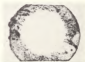
Figure 10. An autoradiogram of an irradiated Si plate after removing thin layers from the central part of the plate (1X).
