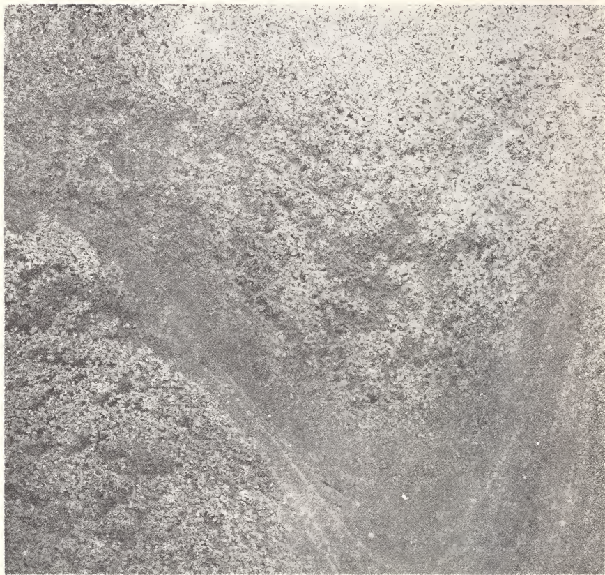
Figure 6. Segregation of tin in aluminum ingot (1X).
