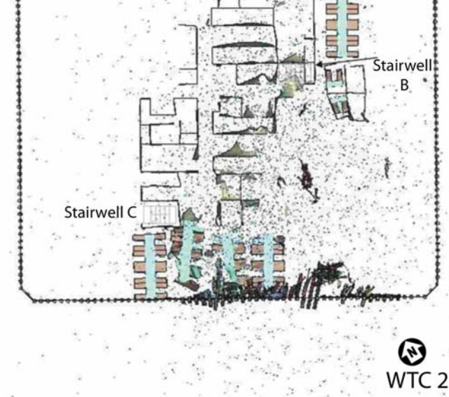
Figure 7–1. WTC 2 damage (computer simulated) at 0.62 s after impact with stairwells superimposed.
