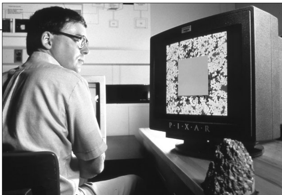
Edward Garboczi, physicist, develops computer models that simulate the microstructure of concrete during the setting process. These models are used to predict concrete performance, strength, and durability.
