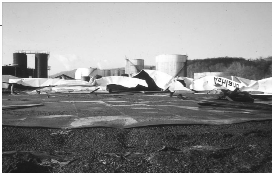
Brittle fracture propagation occurring in tank caused it to rupture and spill its full contents into the neighboring Monongahela River.
