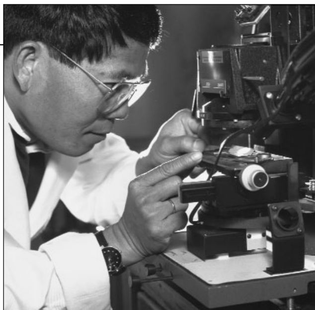
Tinh Nguyen, physical scientist, is using a Fourier transform infrared microscope to study factors affecting the failure of organic protective coatings on steel.
