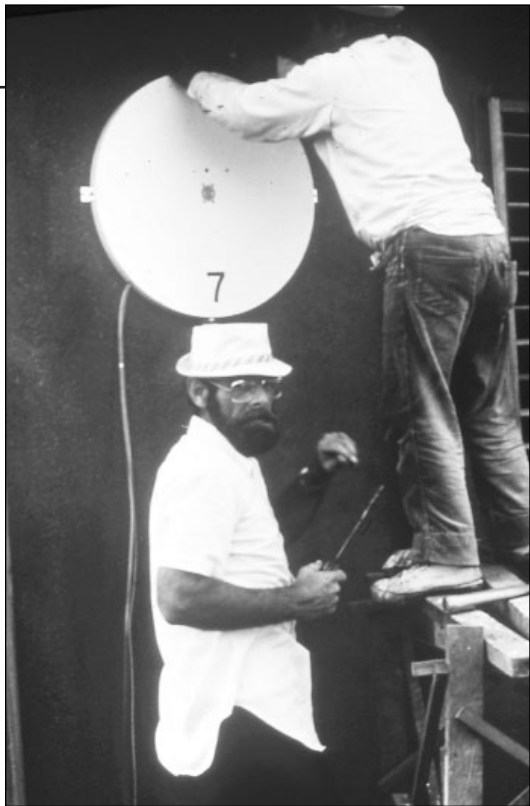
Richard D. Marshall, research structural engineer, with Philippine Weather Bureau technician installing a pressure transducer to one of the wind test houses at the Quezon City, Philippines field test site.
