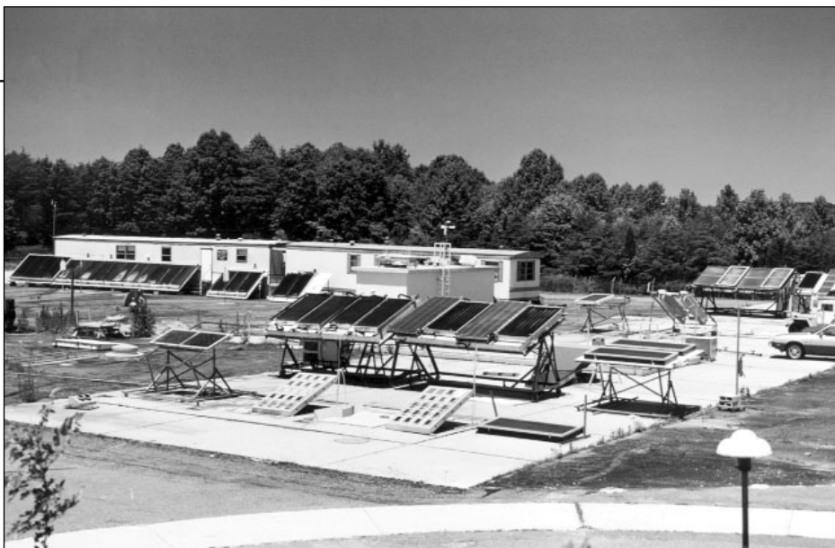
The majority of the experimental work on solar energy equipment took place at the NIST Annex (adjacent to NIST's campus, a former US Army Nike Missile site). The solar equipment, in this photograph, is being used to develop test methods for materials, solar collectors, and solar water heating systems.
