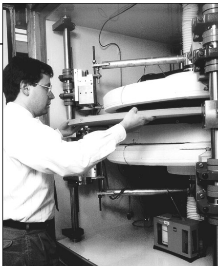
Robert Zarr, research mechanical engineer inserting an insulation sample in NIST's Line Heat Source Guarded Hot Plate, a large-capacity device for measuring the thermal resistance of insulation and other low-density materials up to 380 mm thick and 1 m in diameter. The Hot Plate provides calibrated specimens for guarded hot plates in other laboratories.
