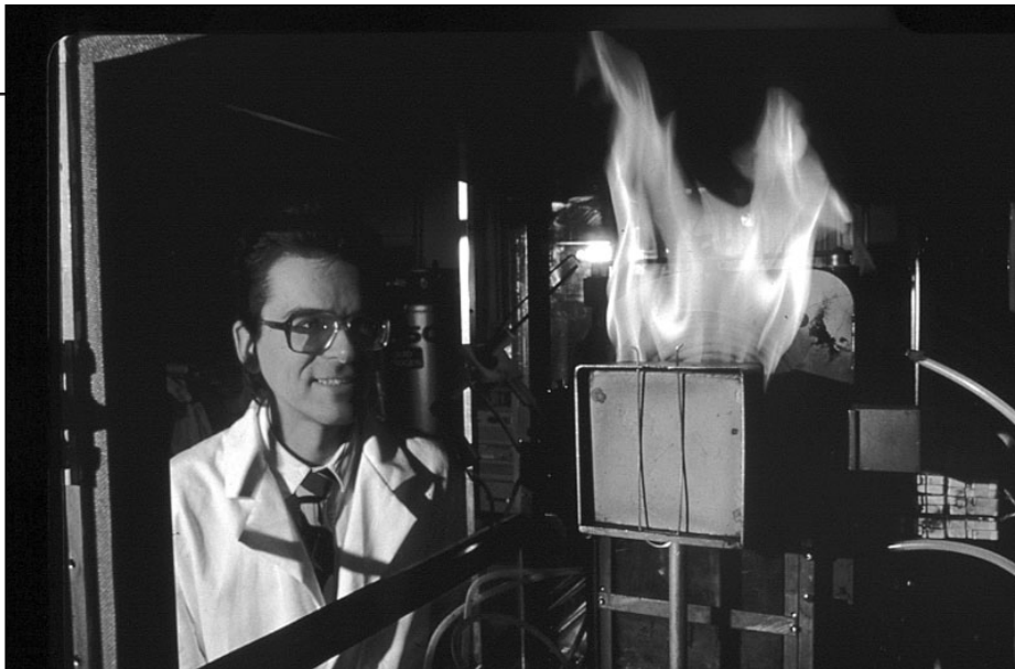
Vytenis Babrauskas, fire protection engineer and developer of the cone calorimeter, is collecting data critical to predicting the fire hazard of a product using a small sample of material. This test replaces time-consuming and expensive full-scale tests. ASTM and ISO adopted a voluntary fire hazard test method based on the instrument.
