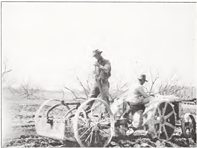
FIG. 3.— Method of collecting gypsite after plowing
