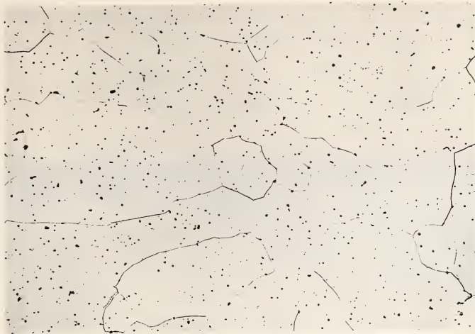
Figure 2. NBS-C1102 brass (cast) near chill-cast face X 50.
