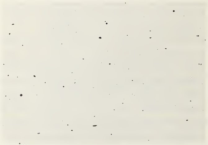
Figure 6. NBS-463 steel, as polished X 200.
