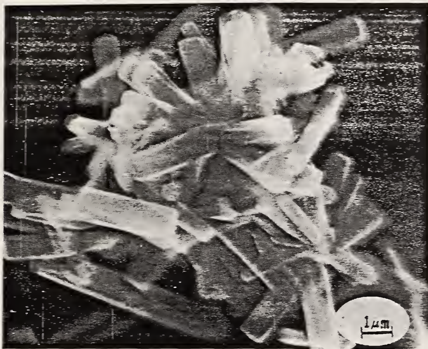
Figure 6. SEM micrograph of Cr-substituted ettringite
