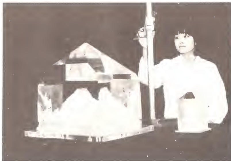
Fig.1. Large KDP crystals developed for laser fusion at ILE. (38cm x 42cm in cross section, 50cm in height)
