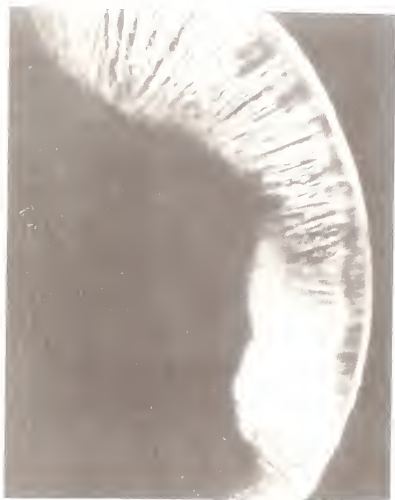
Figure 3. Inclusions near periphery of \text{KCl}(\text{ReO}_4) crystal.
