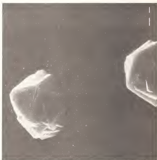
Figure 2. Scanning electron micrographs of diamond particles deposited by the hot filament CVD process on a Si substrate. A 1\mu scale is given by the lower white line in the upper left and lower right micrographs and by the left white line in the upper right and lower left micrographs.
