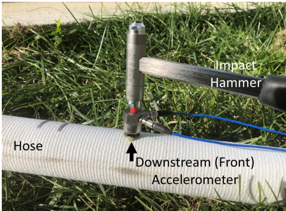
Fig. 19. Impact testing on the downstream (Front) accelerometer using the rubber-tipped impact hammer.
