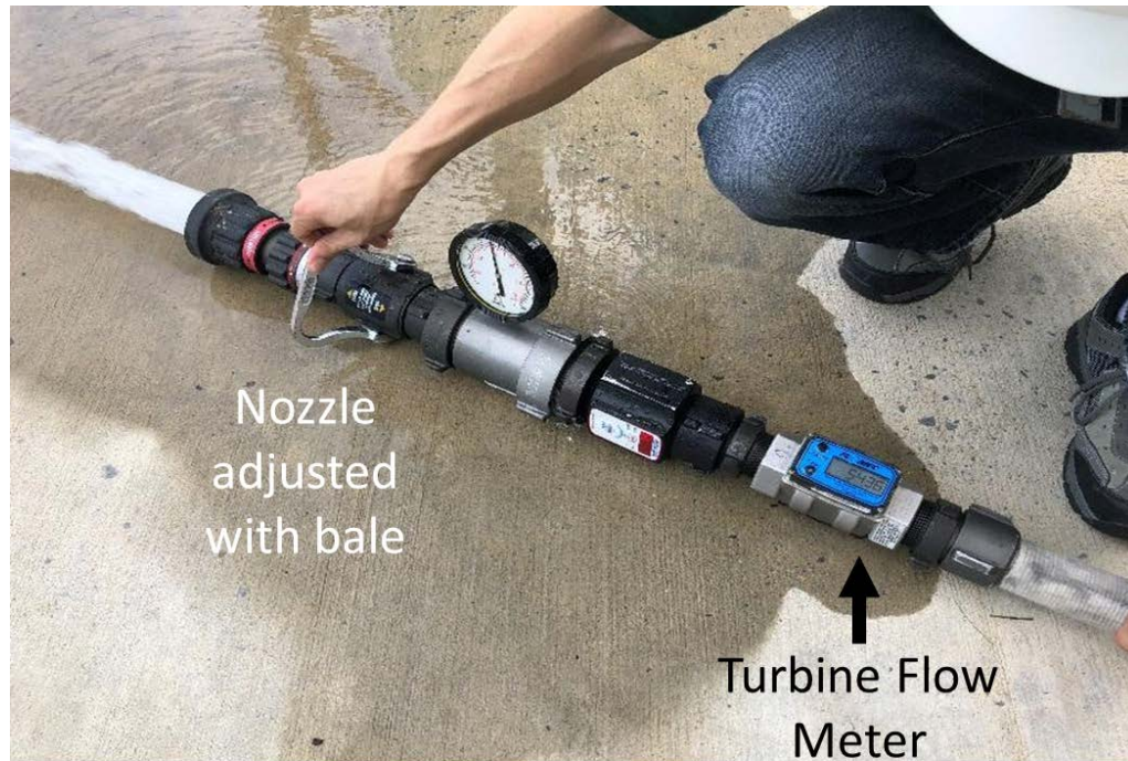
Fig. 9. The flow rate was adjusted for each setting using the nozzle while reading the in-line turbine flow meter.
