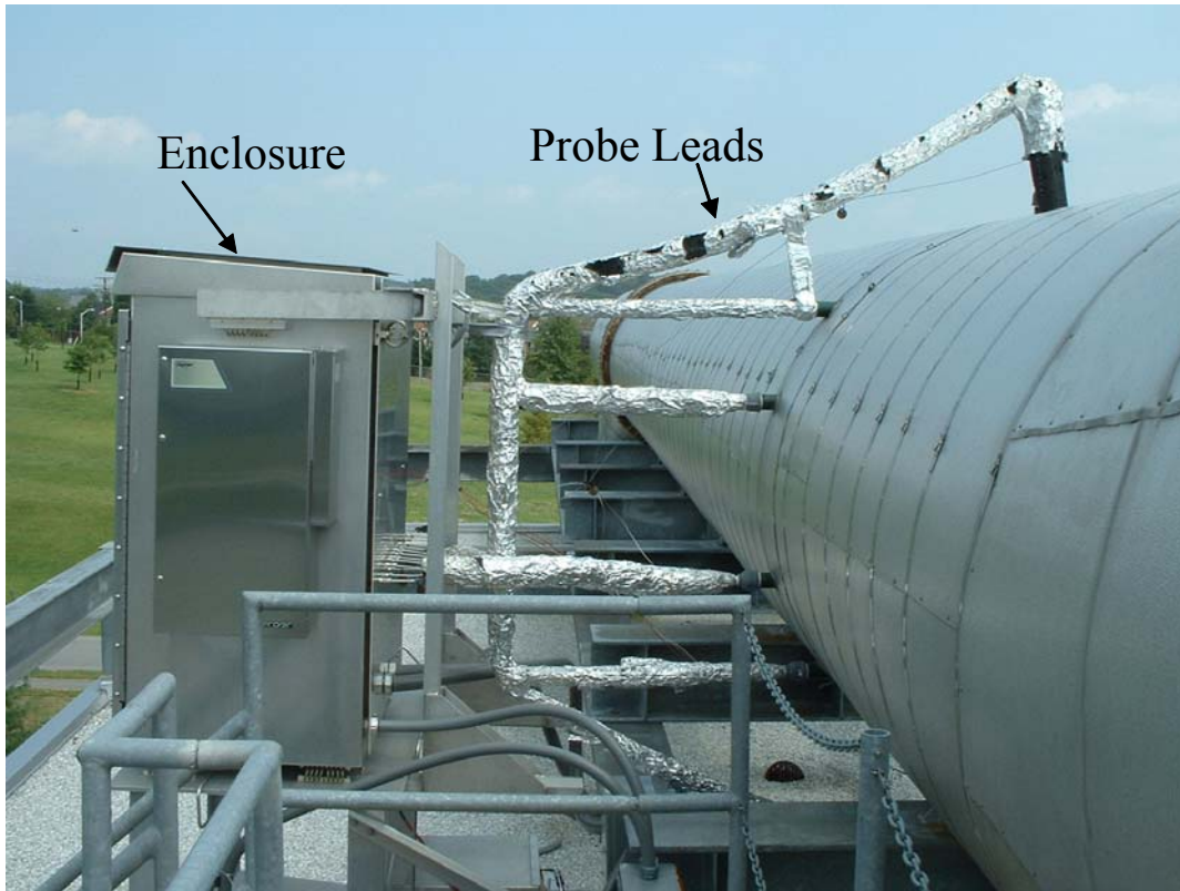
Figure 4 Exhaust duct velocity measurement and gas sampling station.
