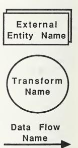
Figure A-2. Data Flow Diagram Symbols
