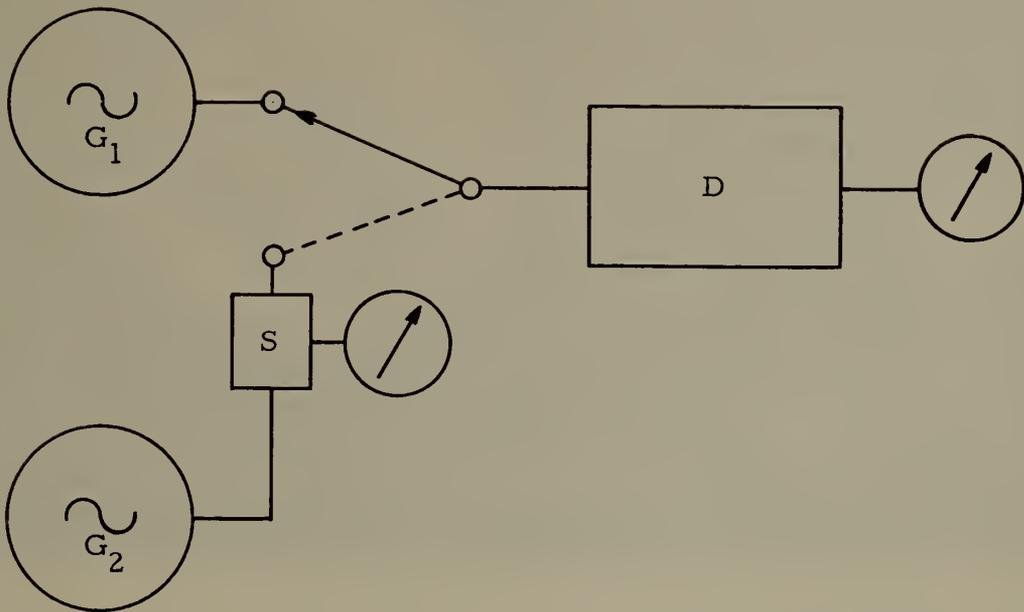
$G_1$  is the rf generator to be calibrated.
