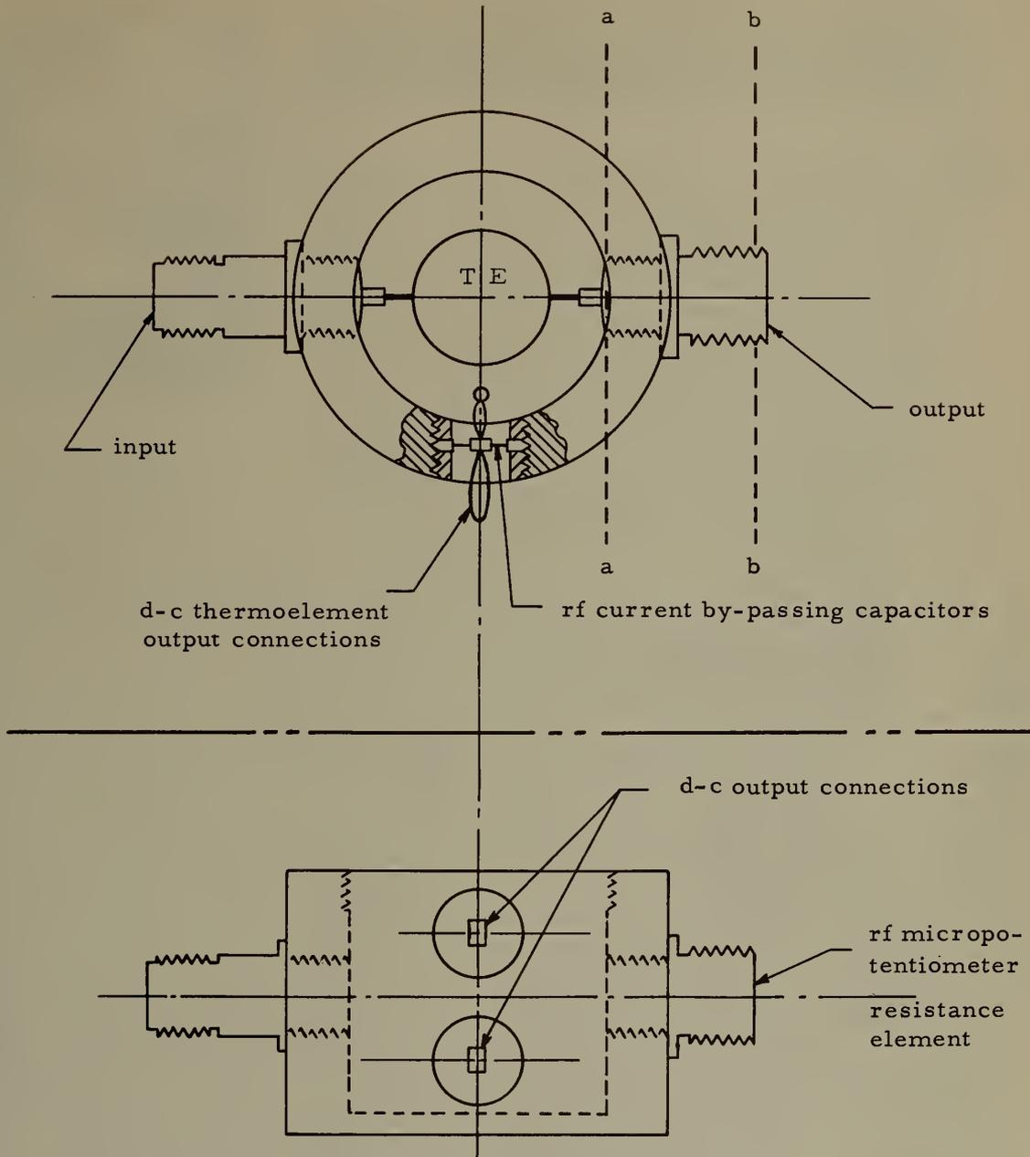
a-a is the plane in which the standardized reference voltage exists.
