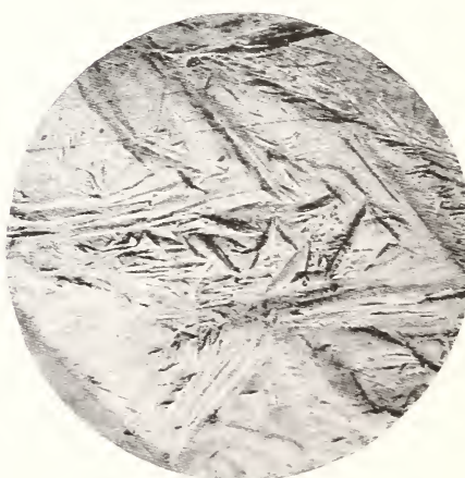
6. C = 0.80 ; Ni = 15.0 . The steel, austenitic at ordinary temperatures, has been rendered martensitic by cooling to -182^{\circ}C in liquid air; unetched
