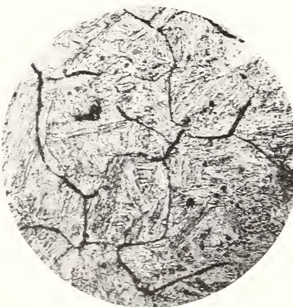
5. C = 0.12 ; Ni = 25.0 . Quenched from 800^{\circ}C ; the outlines of the polyhedral austenite crystals show in the matrix of martensite
