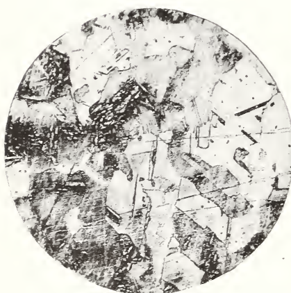
3. C = 0.12 ; Ni = 30.0 . Austenitic structure; invar is very similar in appearance
