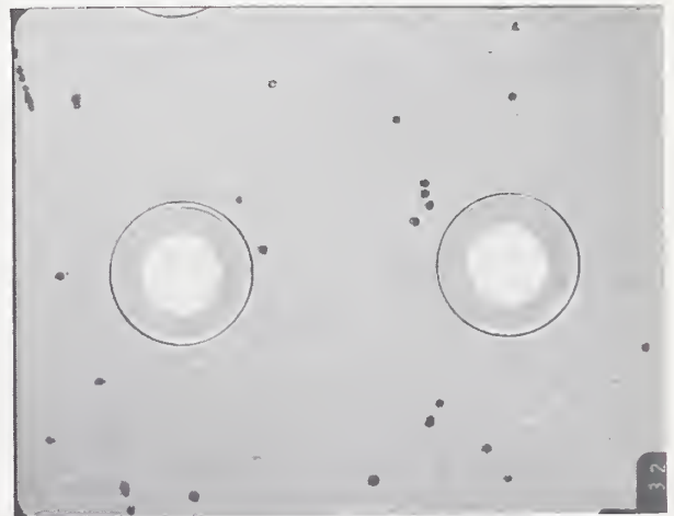
Figure 9. Photomicrograph of typical plasma-etched mesa diode. (The outside diameter of the mesa is about 230 \mu\text{m} .)
