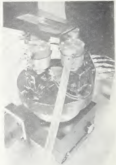
Figure 1. Photograph of probe holder with point contacts for photovoltaic scanning apparatus.
