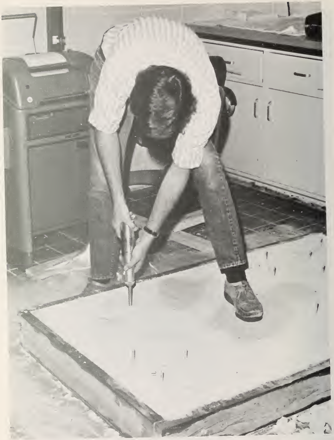
FIGURE 8 Rebound Hammer Test
