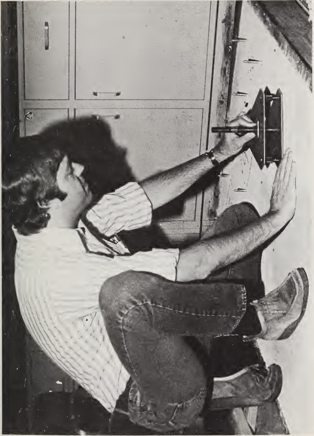
FIGURE 7 A Device Used to Measure the Average Penetration of Three Probes
