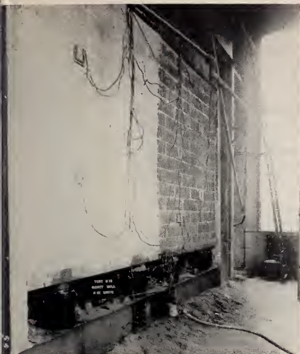
FIGURE 15. Concrete-masonry cavity wall in position for fire test.
