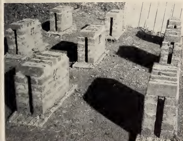
FIGURE 2. Specimens for outdoor weathering of ties.
