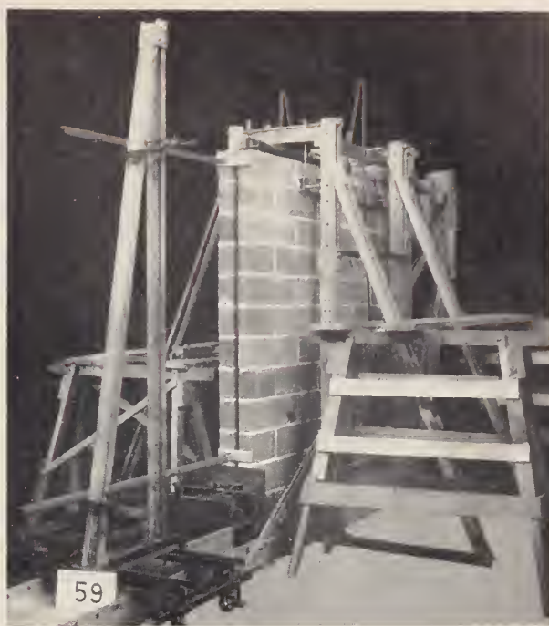
FIGURE 12. Concrete-block cavity wall under racking load. Ties at top restrict vertical motion. Compressometers measure horizontal deformation.
