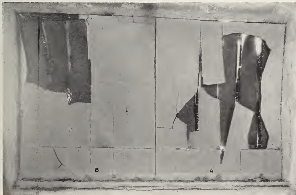
FIGURE 5. Exposed side of asbestos-cement sheet-faced partition, no insulation, after failure under fire and load. Test 1.
