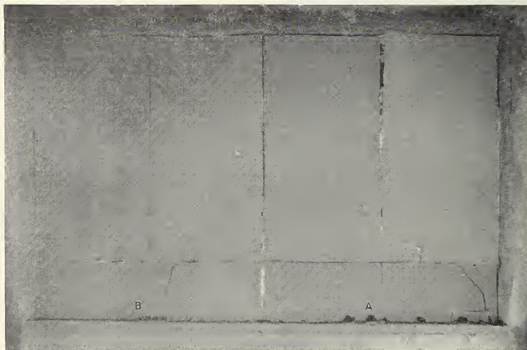
FIGURE 8. Partition with mineral-wool fill and gypsum-board strips on edges of studs. Fire-exposed face after 1 hr 32 min. — Test 6.
