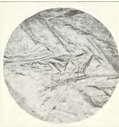
6. C=0.80; Ni=15.0. The steel, austenitic at ordinary temperatures, has been rendered martensitic by cooling to -182° C. in liquid air; unetched.
