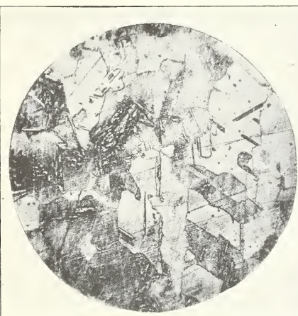
3. C=0.12; Ni=30.0. Austenitic structure; invar is very similar in appearance.
