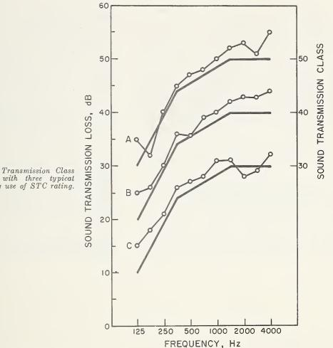
FIGURE 2. Sound Transmission Class (STC) contours with three typical spectra illustrating use of STC rating.
