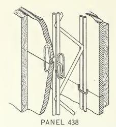
PANEL 438. 2½-by ½-in. steel studs placed 16 in. on centers with stud shoes wire-tied to steel runners. Galvanized wire clips attached to studs on both sides, held ½-in. plain gypsum lath, joined with sheet metal clips, ½-in. gypsum vermiculite plaster, and ½-in. white-coat finish. (Sheet metal clip similar to "D" clip, p. 44 of BMS Report 144.)
