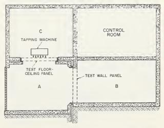
Vertical section of NBS sound transmission FIGURE 1. facilities.
