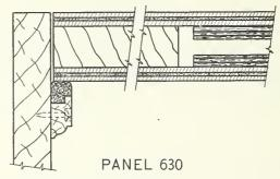
PANEL 630. 2½-by 36-by 84-in. wooden door with a 1½-in.-thick core; on each side, ½-in. seven-ply panels with ½-in. sponge rubber centers; panels backed with laminated layer of damping material. Corrugated sponge rubber gaskets similar to those of panel 624 were used, and a sponge rubber drop closure was installed in bottom of the door. The door was completely sealed around the edges on the side opposite the gaskets with a soft clay caulking compound.
