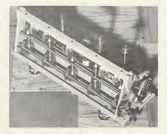
FIGURE 3. Tapping machine used for generating sound field for impact sound transmission measurements. The five 0.5 kg hammers fall 4 cm to the floor and produce 10 impacts per second.
