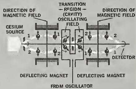
A schematic of an atomic beam spectrometer. The trajectories are drawn for those atoms whose magnetic moments are "flipped" in the transition region.
