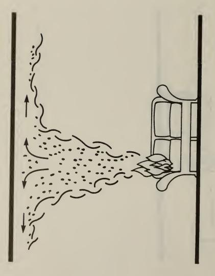
Figure 3. The plume-ceiling interaction.
