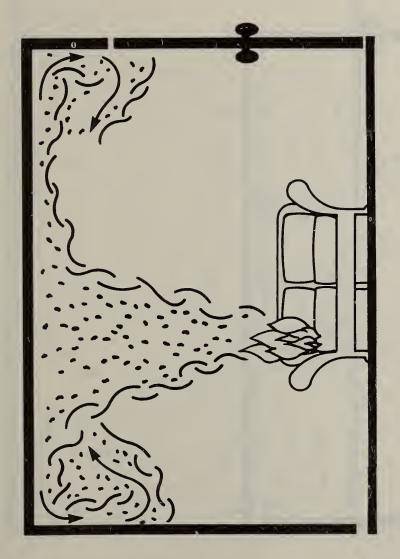
Figure 4. Ceiling jet-wall interactions.
