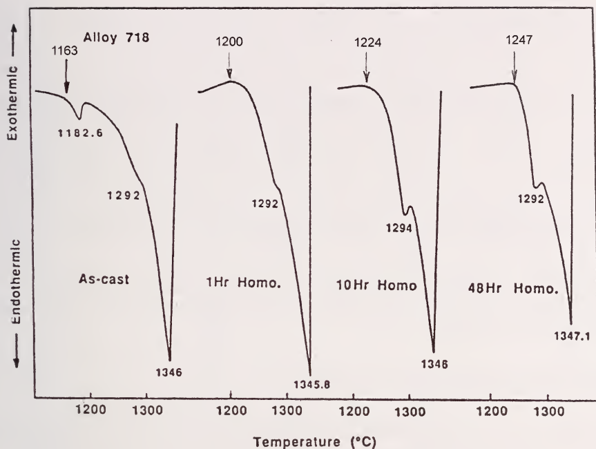
Figure 3.7. DTA signal for Inconel 718 showing the effect of annealing time [91Cao]. With annealing, the (\text{Fe,Cr})_2\text{Nb} Laves phase dissolves and the onset of melting increases from 1163^\circ\text{C} to 1247^\circ\text{C} .
