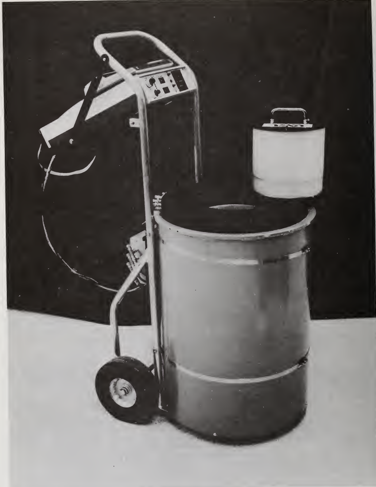
Figure 3 Photograph of AWCC system complete with detector body and cart, electronics package and HP-97 calculator for automated data readout and analysis.
