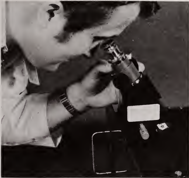
Figure 2. Inspecting the integrity of a fiber-optic seal.
