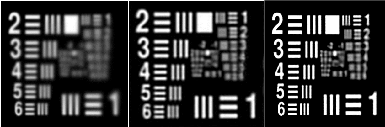
Figure 6. In 512x512 resolution chart image, stabilized backward time-marching with \varepsilon = 3.5 \times 10^{-4} , p = 2.5 , competently recovers vertical sequence of numbers near image right edge in relatively little computing time, while the Van Cittert iteration is computationally impractical on large problems.
