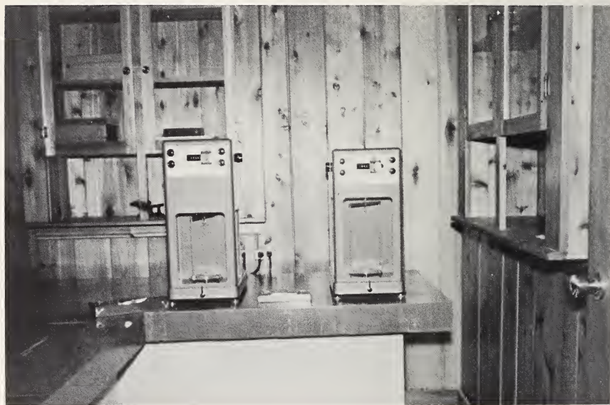
Two Mettler balances. Two balances of 100 gram and 1000 gram capacities, on a vibrationless table.
