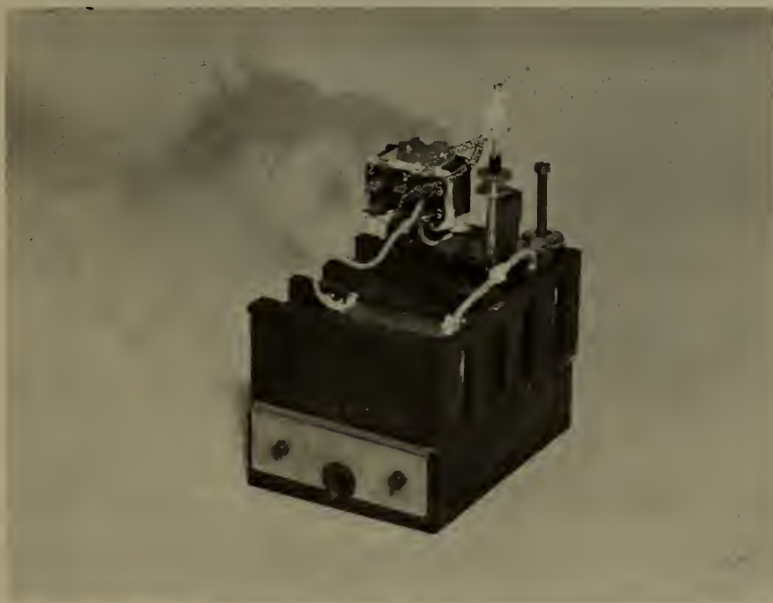
Figure 10. Controlled-temperature cell block for spectrophotometric measurements.
