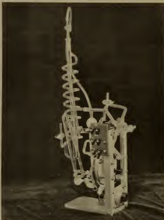
Figure 13. Conductometric cell for the determination of small amounts of water in a gas stream.
